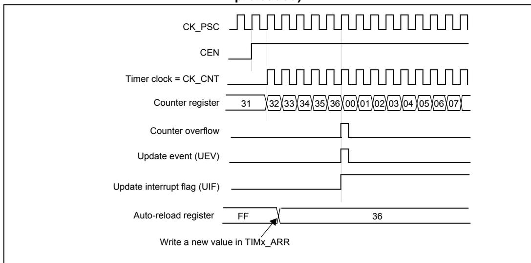
**Figure 47. Counter timing diagram, update event when ARPE=1 (TIMx\_ARR preloaded)**
