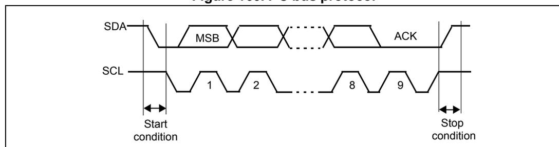
Acknowledge may be enabled or disabled by software. The I<sup>2</sup>C interface addresses (dual addressing 7-bit/ 10-bit and/or general call address) can be selected by software.
