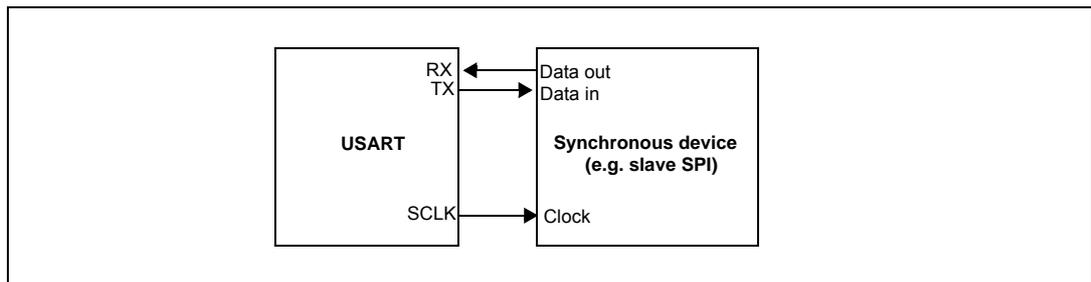
Figure 179. USART data clock timing diagram (M=0)
