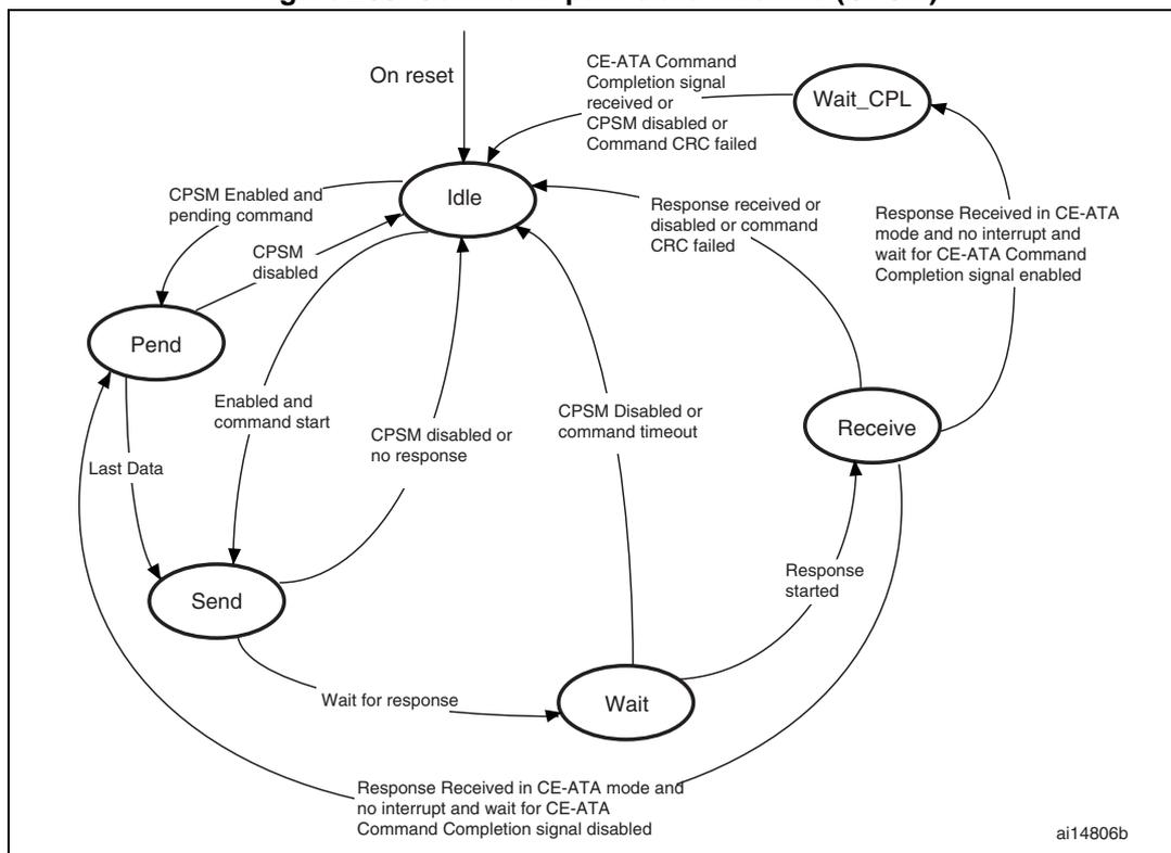
When the Wait state is entered, the command timer starts running. If the timeout is reached before the CPSM moves to the Receive state, the timeout flag is set and the Idle state is entered.
