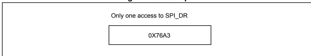
For transmission, each time an MSB is written to SPI\_DR, the TXE flag is set and its interrupt, if allowed, is generated to load SPI\_DR with the new value to send. This takes place even if 0x0000 have not yet been sent because it is done by hardware.
