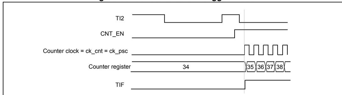
**Slave mode: external clock mode 2 + trigger mode**
