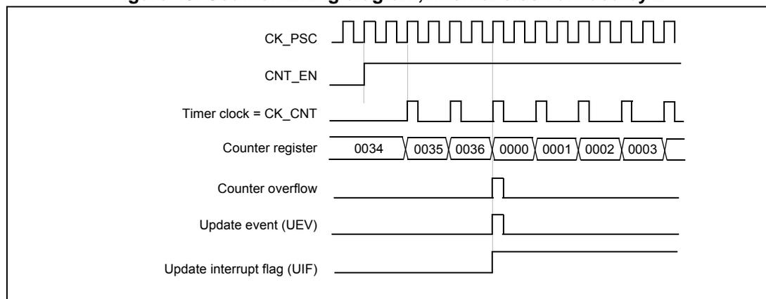
**Figure 44. Counter timing diagram, internal clock divided by 4**
