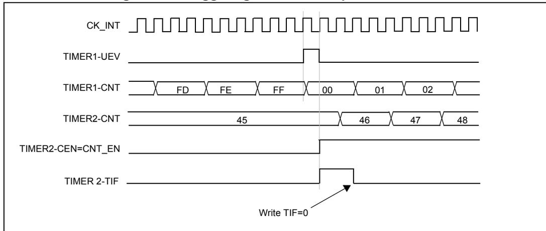
As in the previous example, you can initialize both counters before starting counting. [Figure 131](#) shows the behavior with the same configuration as in [Figure 162](#) but in trigger mode instead of gated mode (SMS=110 in the TIM2\_SMCR register).
