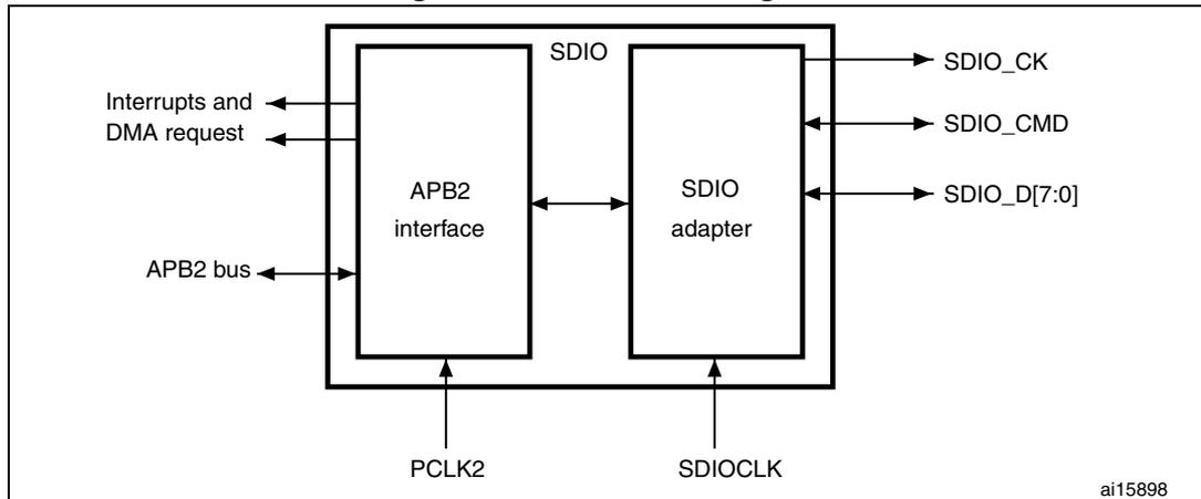
By default SDIO\_D0 is used for data transfer. After initialization, the host can change the databus width.
