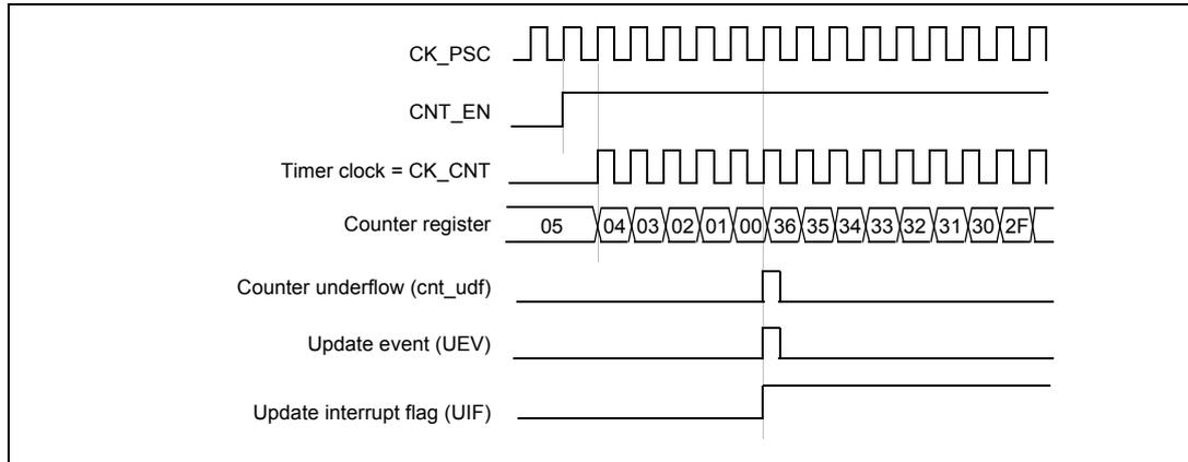
**Figure 49. Counter timing diagram, internal clock divided by 2**
