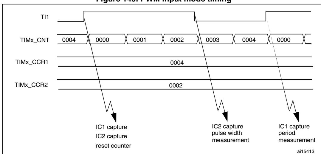
1. The PWM input mode can be used only with the TIMx\_CH1/TIMx\_CH2 signals due to the fact that only TI1FP1 and TI2FP2 are connected to the slave mode controller.
