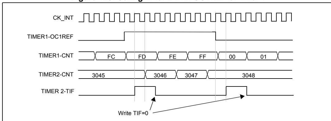
In the example in [Figure 162](#), the Timer 2 counter and prescaler are not initialized before being started. So they start counting from their current value. It is possible to start from a given value by resetting both timers before starting Timer 1. You can then write any value you want in the timer counters. The timers can easily be reset by software using the UG bit in the TIMx\_EGR registers.
