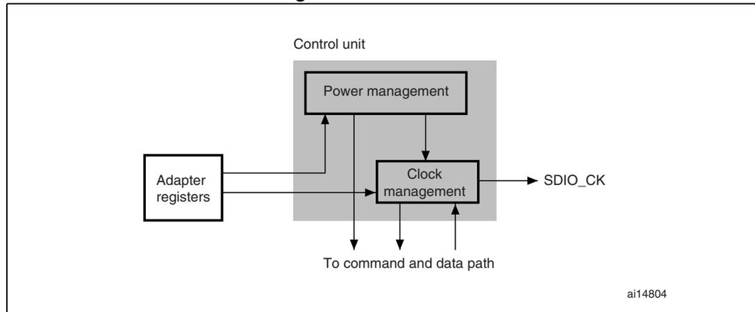
The control unit is illustrated in [Figure 236](#). It consists of a power management subunit and a clock management subunit.
