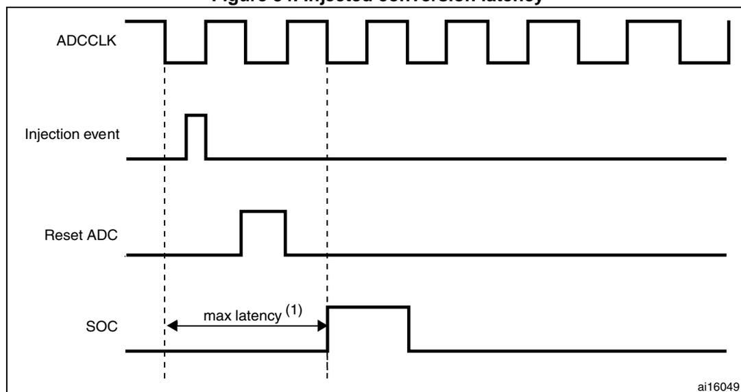
1. The maximum latency value can be found in the electrical characteristics of the STM32F411xC/E datasheets.
