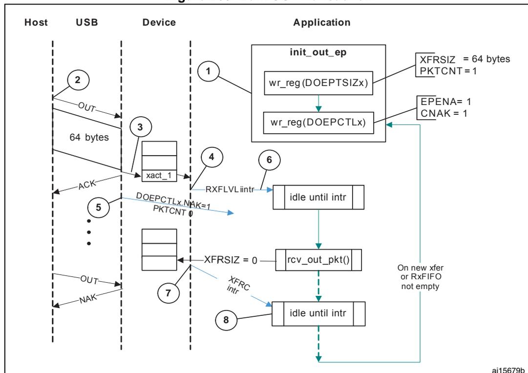
After a SetConfiguration/SetInterface command, the application initializes all OUT endpoints by setting CNAK = 1 and EPENA = 1 (in OTG\_FS\_DOEPTLx), and setting a suitable XFRSIZ and PKTCNT in the OTG\_FS\_DOEPTSIzX register.
