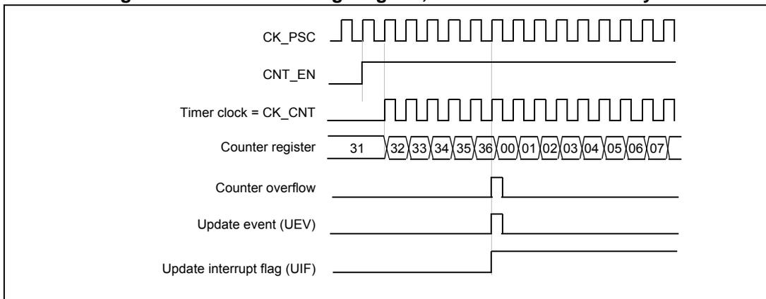
**Figure 138. Counter timing diagram, internal clock divided by 2**
