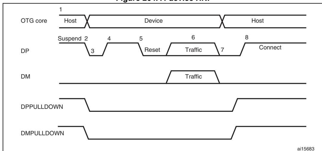
1. DPPULLDOWN = signal from core to PHY to enable/disable the pull-down on the DP line inside the PHY.
