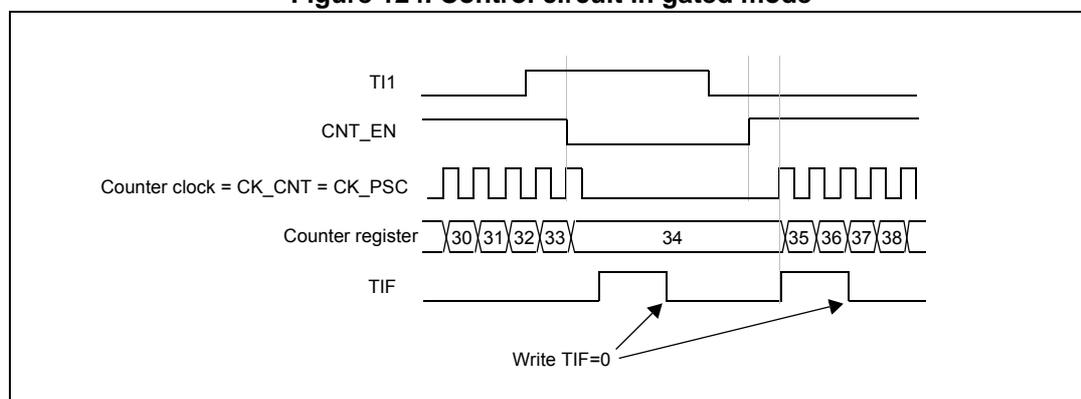
1. The configuration "CCxP=CCxNP=1" (detection of both rising and falling edges) does not have any effect in gated mode because gated mode acts on a level and not on an edge.
