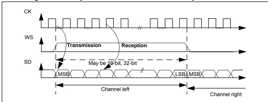
Figure 220. LSB Justified 24-bit frame length with CPOL = 0
