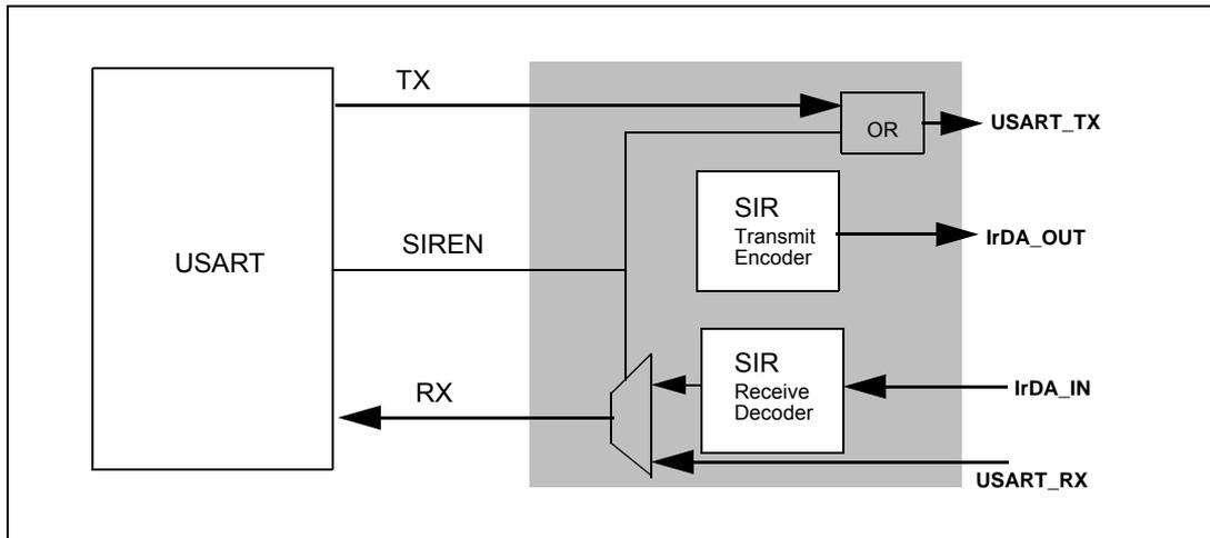
**Figure 185. IrDA data modulation (3/16) -Normal mode**
