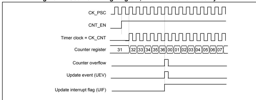
**Figure 43. Counter timing diagram, internal clock divided by 2**
