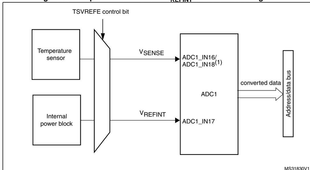
1.  $V_{SENSE}$  is input to ADC1\_IN18
