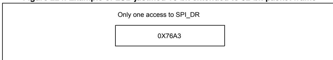
In transmission mode, when TXE is asserted, the application has to write the data to be transmitted (in this case 0x76A3). The 0x000 field is transmitted first (extension on 32-bit). TXE is asserted again as soon as the effective data (0x76A3) is sent on SD.
