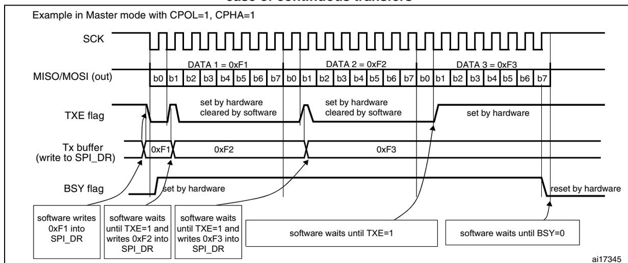
**Figure 202. TXE/BSY in Slave transmit-only mode (BIDIMODE=0 and RXONLY=0) in the case of continuous transfers**
