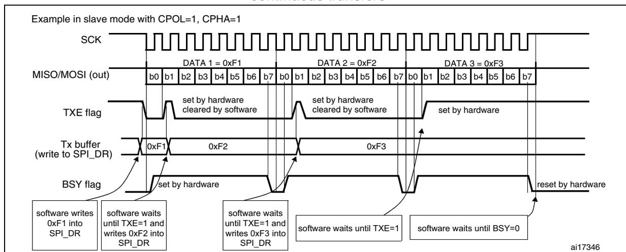
**Bidirectional transmit procedure (BIDIMODE=1 and BIDIOE=1)**
