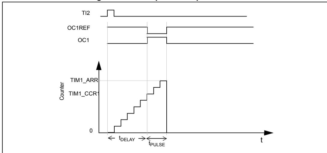
For example you may want to generate a positive pulse on OC1 with a length of  $t_{PULSE}$  and after a delay of  $t_{DELAY}$  as soon as a positive edge is detected on the TI2 input pin.
