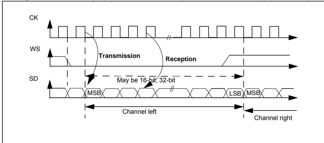
Data are latched on the falling edge of CK (for the transmitter) and are read on the rising edge (for the receiver). The WS signal is also latched on the falling edge of CK.
