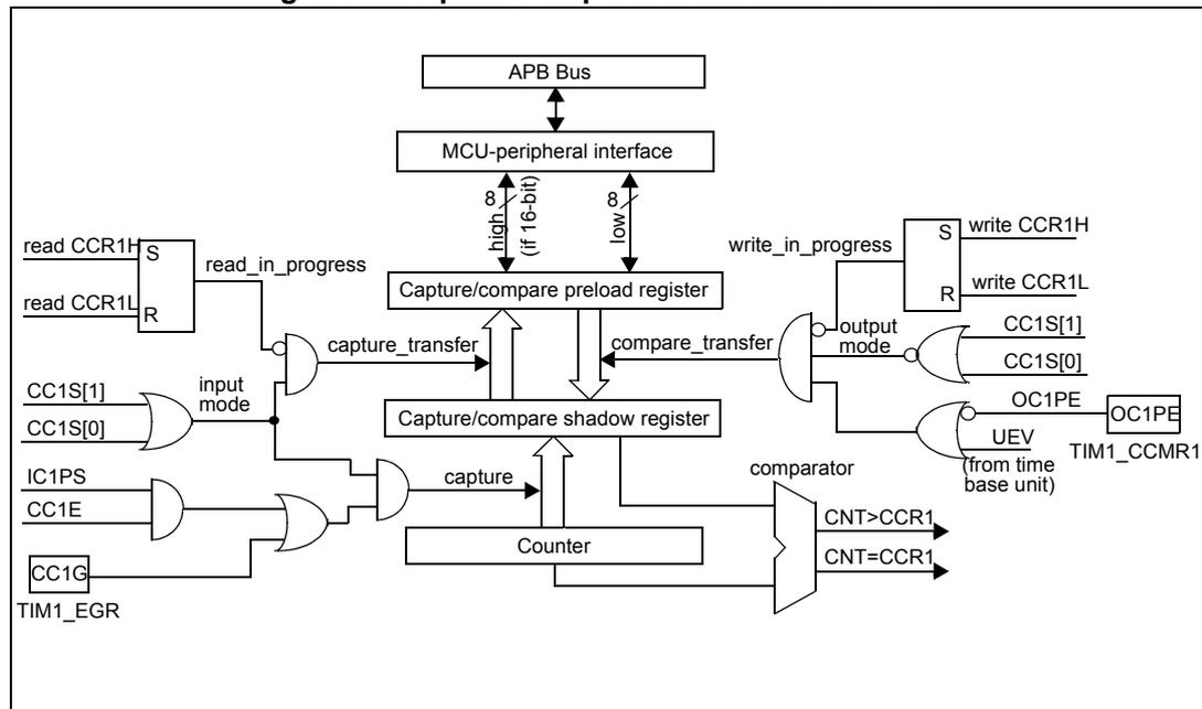
Figure 67. Output stage of capture/compare channel (channel 1 to 3)
