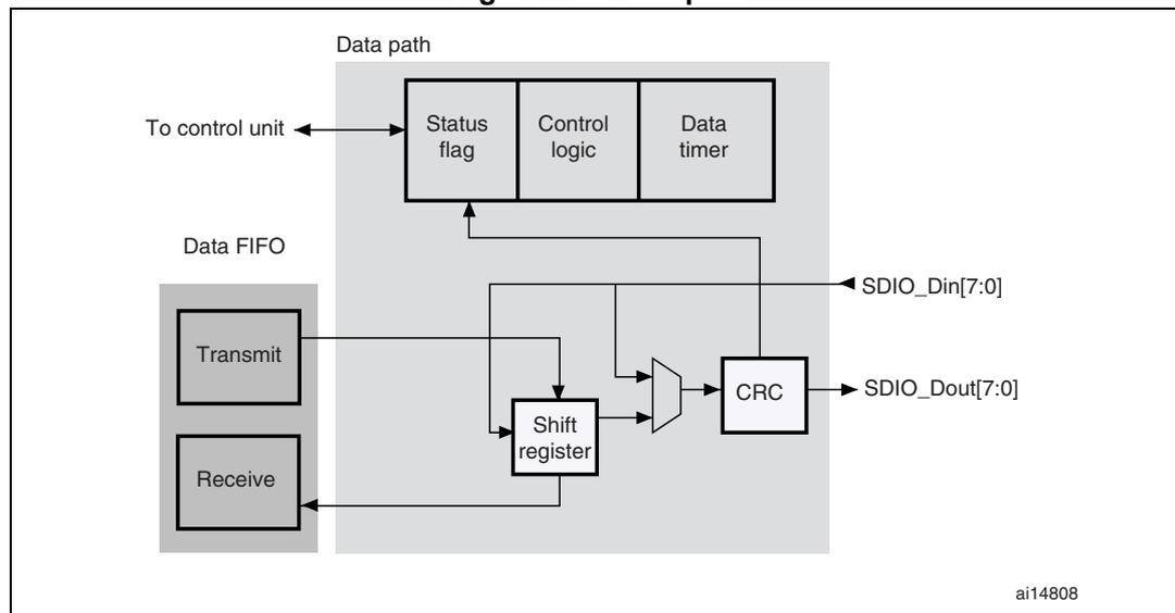
The card databus width can be programmed using the clock control register. If the 4-bit wide bus mode is enabled, data is transferred at four bits per clock cycle over all four data signals (SDIO\_D[3:0]). If the 8-bit wide bus mode is enabled, data is transferred at eight bits per clock cycle over all eight data signals (SDIO\_D[7:0]). If the wide bus mode is not enabled, only one bit per clock cycle is transferred over SDIO\_D0.
