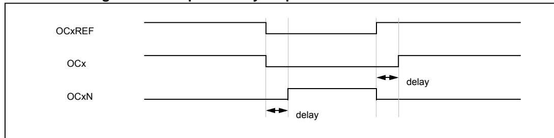
**Figure 74. Dead-time waveforms with delay greater than the negative pulse.**
