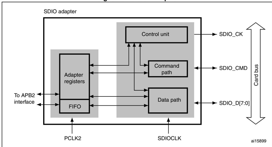
The SDIO adapter is a multimedia/secure digital memory card bus master that provides an interface to a multimedia card stack or to a secure digital memory card. It consists of five subunits:
