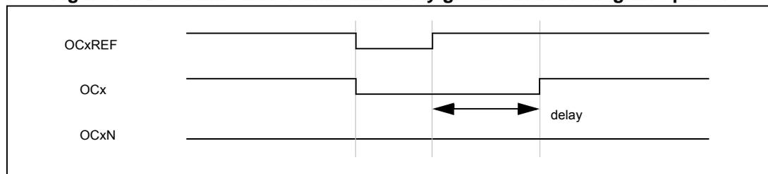
**Figure 75. Dead-time waveforms with delay greater than the positive pulse.**
