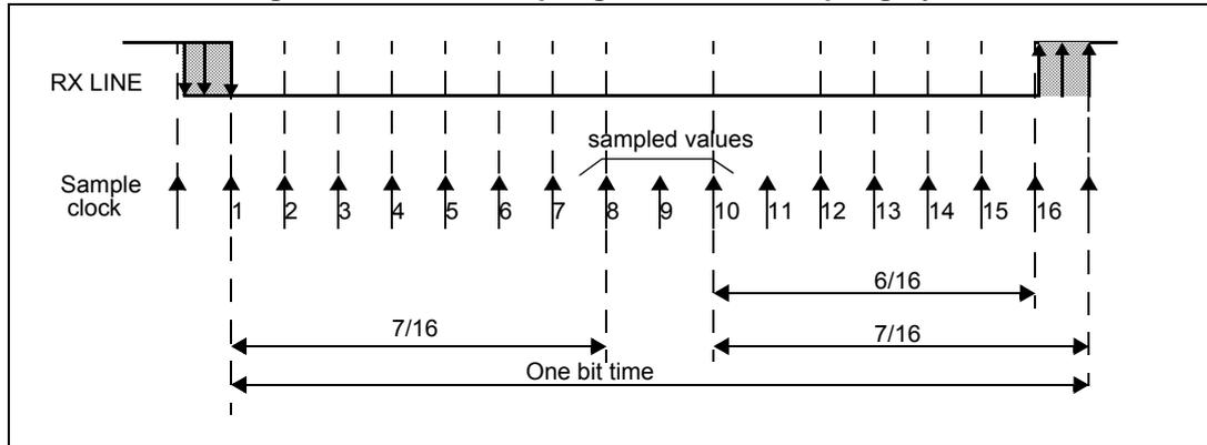
**Figure 173. Data sampling when oversampling by 8**
