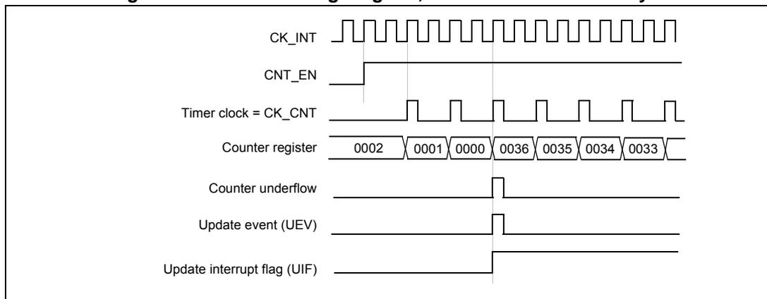
**Figure 98. Counter timing diagram, internal clock divided by 4**
