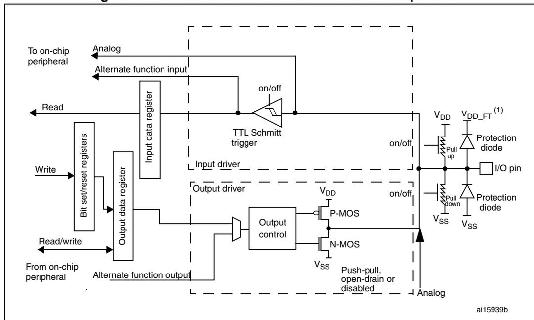
1. V<sub>DD\_FT</sub> is a potential specific to five-volt tolerant I/Os and different from V<sub>DD</sub>.
