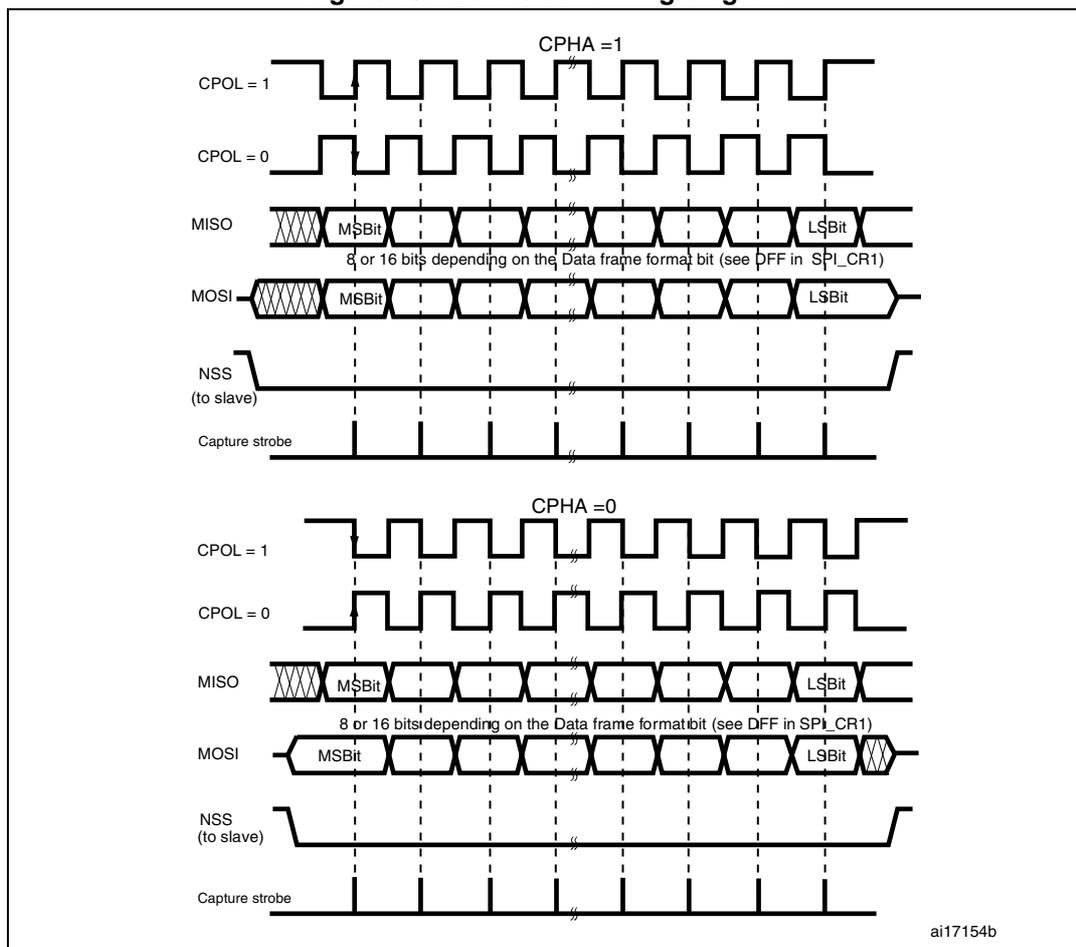
1. These timings are shown with the LSBFIRST bit reset in the SPI\_CR1 register.
