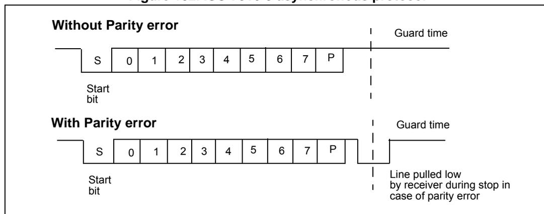
When connected to a Smartcard, the TX output of the USART drives a bidirectional line that is also driven by the Smartcard. The TX pin must be configured as open-drain.
