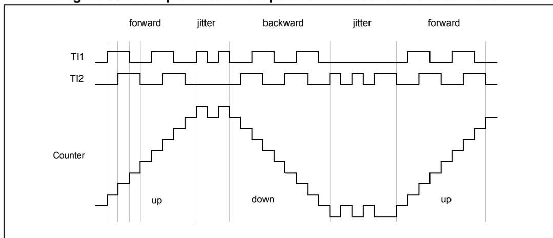
Figure 81 gives an example of counter behavior when TI1FP1 polarity is inverted (same configuration as above except CC1P='1').
