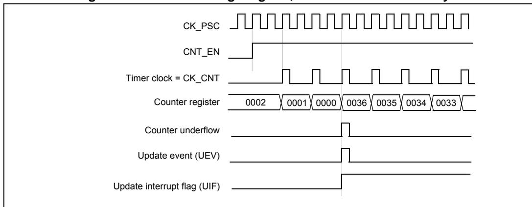
**Figure 50. Counter timing diagram, internal clock divided by 4**
