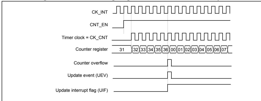
**Figure 91. Counter timing diagram, internal clock divided by 2**
