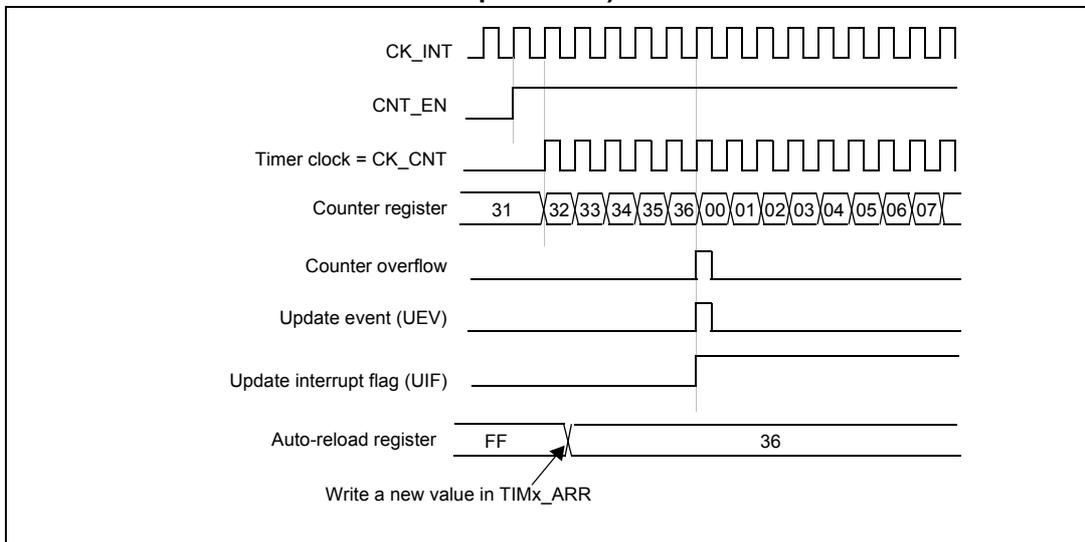
**Figure 95. Counter timing diagram, Update event when ARPE=1 (TIMx\_ARR preloaded)**
