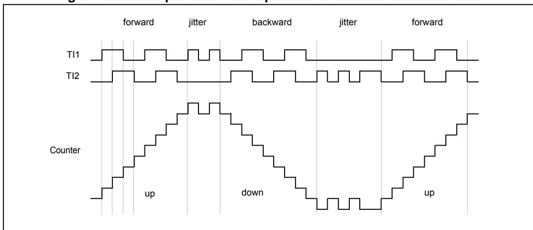
Figure 122 gives an example of counter behavior when TI1FP1 polarity is inverted (same configuration as above except CC1P=1).
