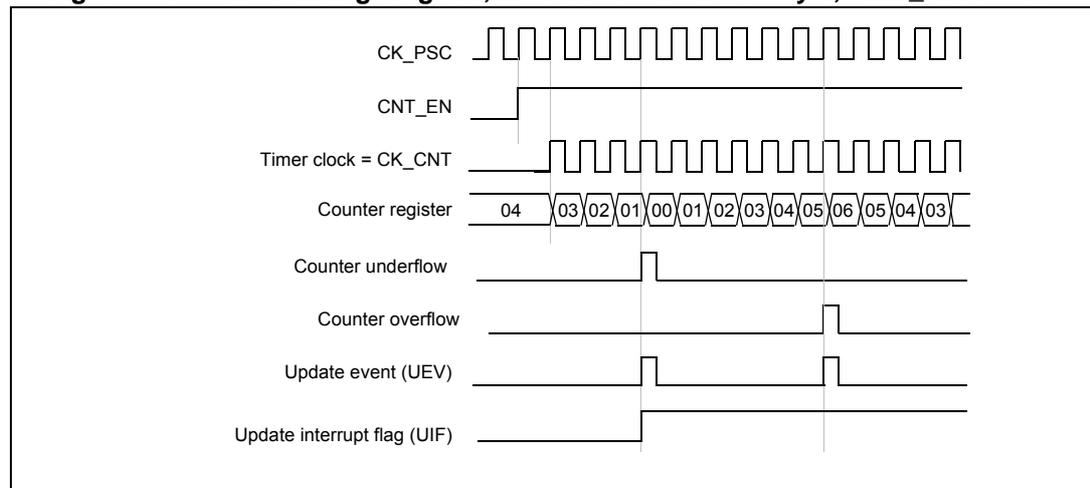
1. Here, center-aligned mode 1 is used (for more details refer to [Section 12.4: TIM1 registers on page 278](#)).
