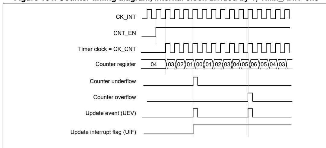
1. Here, center-aligned mode 1 is used (for more details refer to [Section 13.4.1: TIMx control register 1 \(TIMx\\_CR1\) on page 342](#)).
