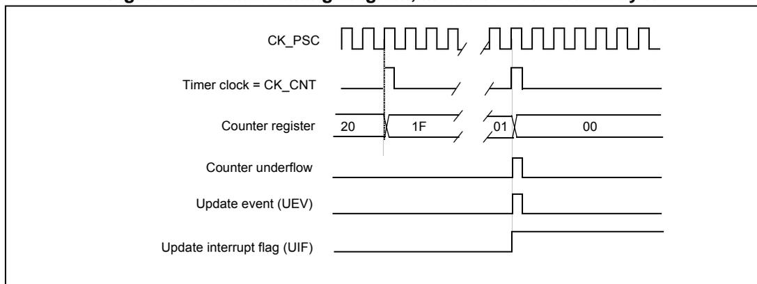
**Figure 57. Counter timing diagram, update event with ARPE=1 (counter underflow)**
