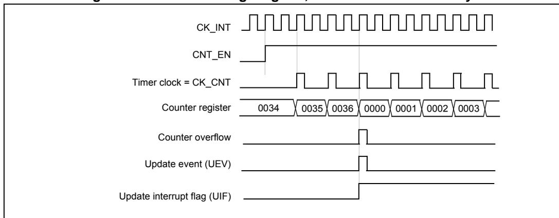
**Figure 92. Counter timing diagram, internal clock divided by 4**
