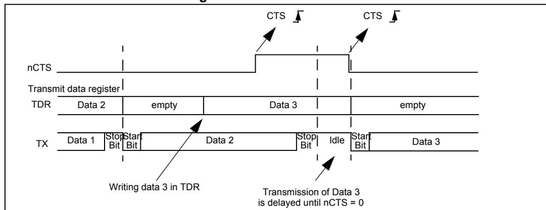
Note: **Special behavior of break frames:** when the CTS flow is enabled, the transmitter does not check the nCTS input state to send a break.
