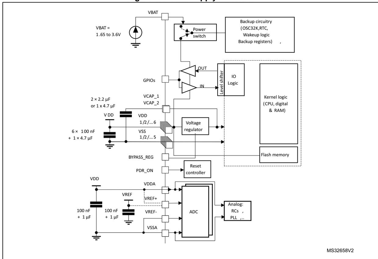
1. V<sub>DDA</sub> and V<sub>SSA</sub> must be connected to V<sub>DD</sub> and V<sub>SS</sub>, respectively.
