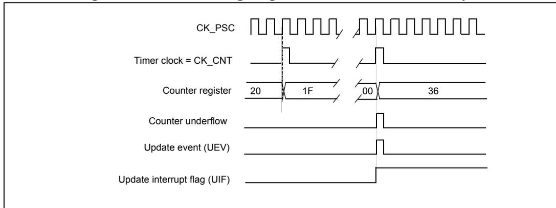
**Figure 52. Counter timing diagram, update event when repetition counter is not used**
