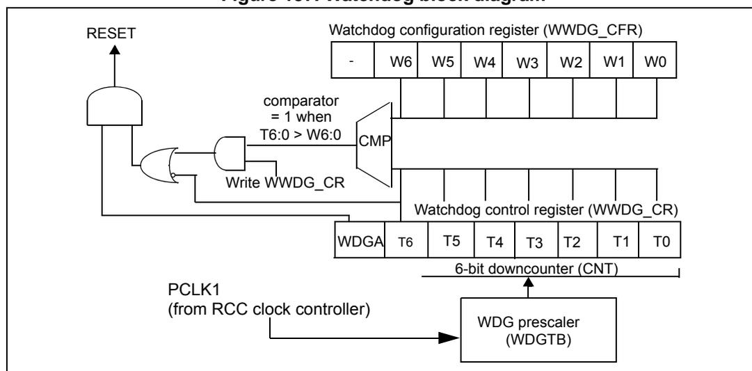
The application program must write in the WWDG\_CR register at regular intervals during normal operation to prevent an MCU reset. This operation must occur only when the counter value is lower than the window register value. The value to be stored in the WWDG\_CR register must be between 0xFF and 0xC0:
