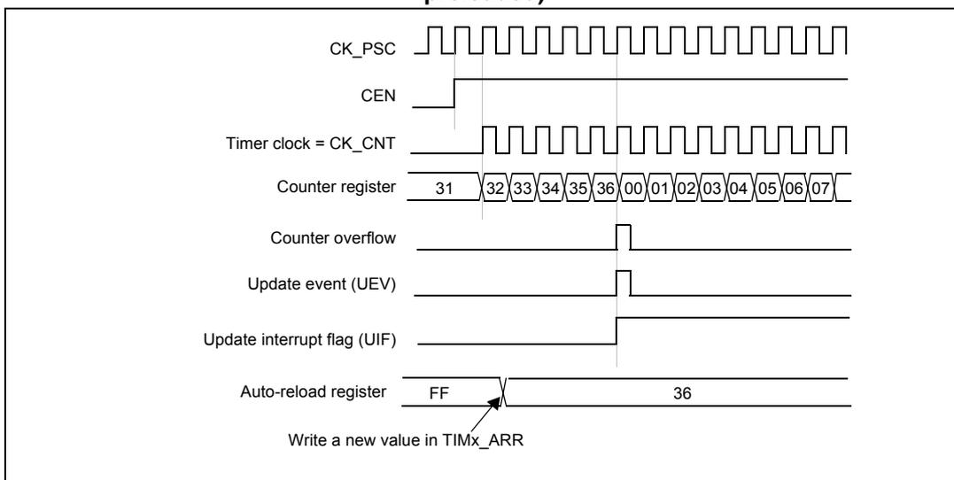
**Figure 142. Counter timing diagram, update event when ARPE=1 (TIMx\_ARR preloaded)**
