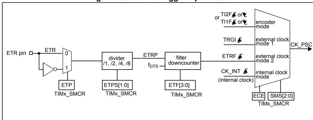
For example, to configure the upcounter to count each 2 rising edges on ETR, use the following procedure:
