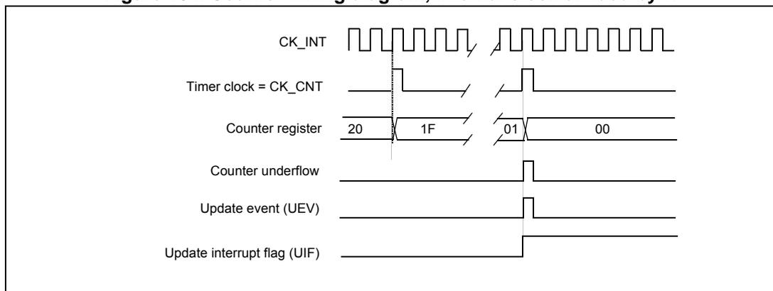
**Figure 105. Counter timing diagram, Update event with ARPE=1 (counter underflow)**
