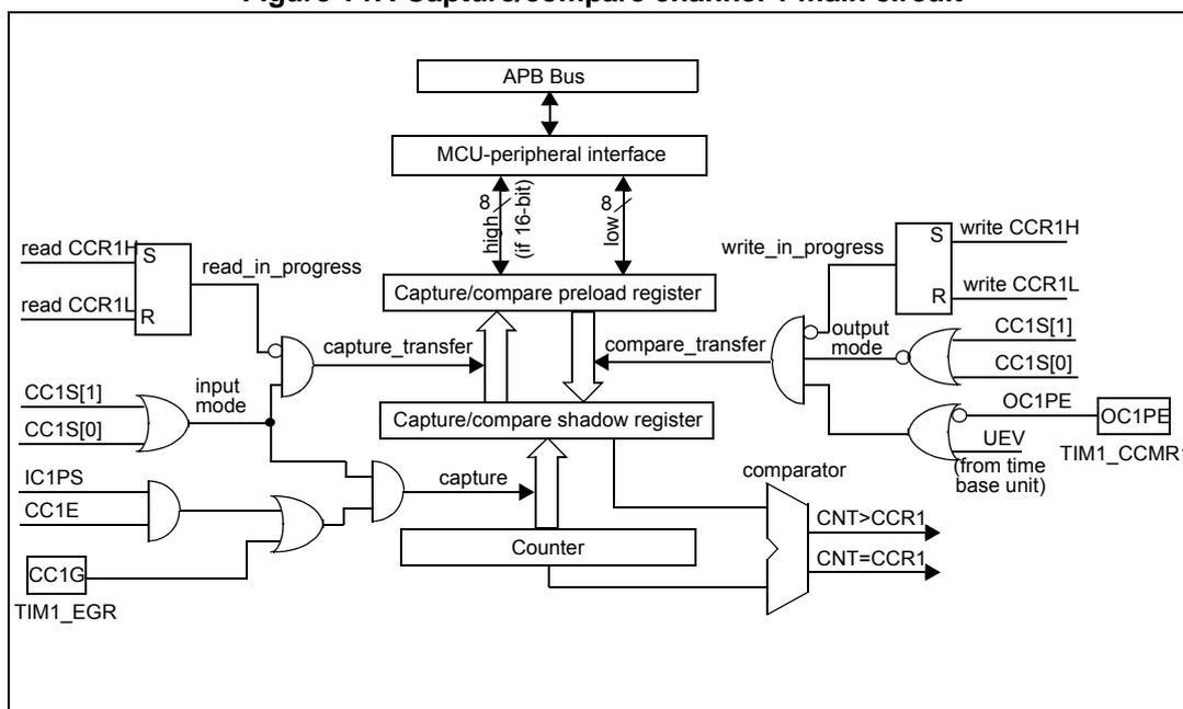
Figure 148. Output stage of capture/compare channel (channel 1)
