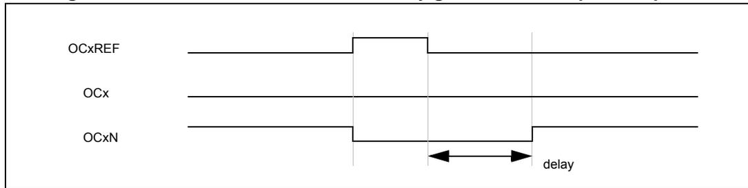
The dead-time delay is the same for each of the channels and is programmable with the DTG bits in the TIMx\_BDTR register. Refer to [Section 12.4.18: TIM1 break and dead-time register \(TIMx\\_BDTR\) on page 300](#) for delay calculation.
