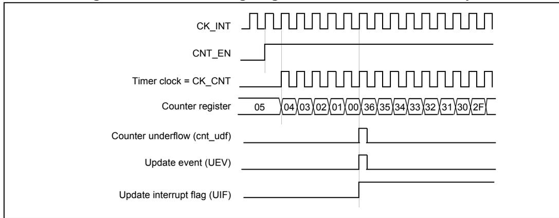
**Figure 97. Counter timing diagram, internal clock divided by 2**
