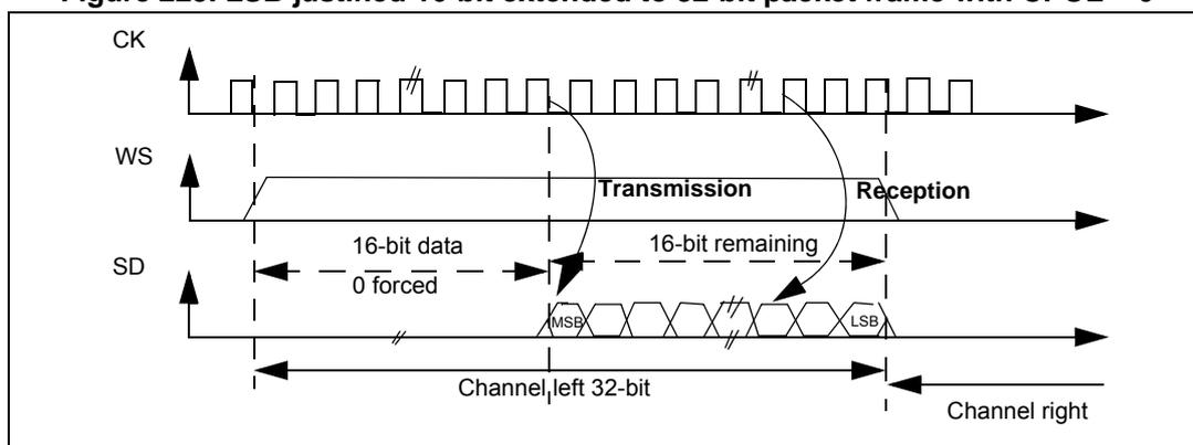
When 16-bit data frame extended to 32-bit channel frame is selected during the I<sup>2</sup>S configuration phase, Only one access to SPI\_DR is required. The 16 remaining bits are forced by hardware to 0x0000 to extend the data to 32-bit format. In this case it corresponds to the half-word MSB.
