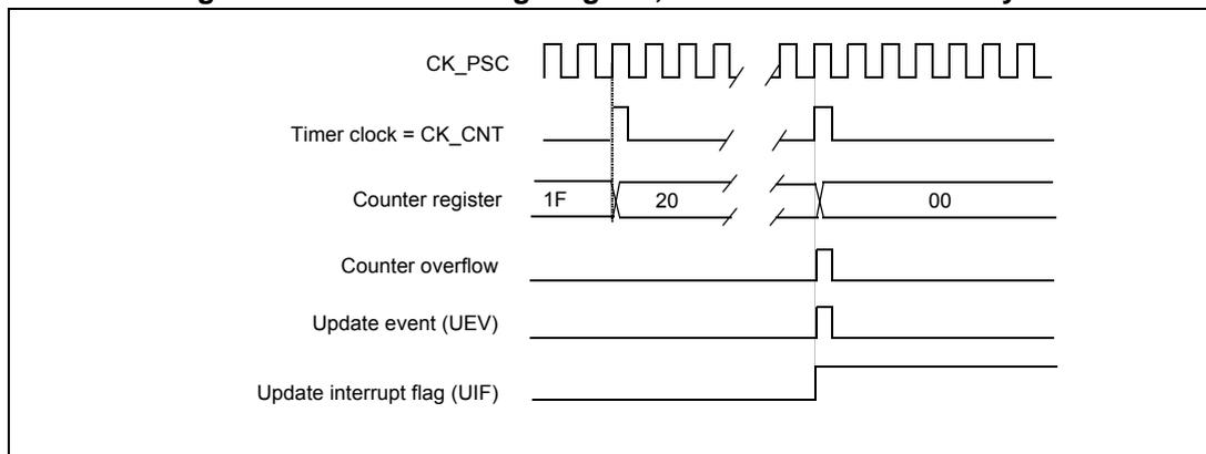
**Figure 46. Counter timing diagram, update event when ARPE=0 (TIMx\_ARR not preloaded)**
