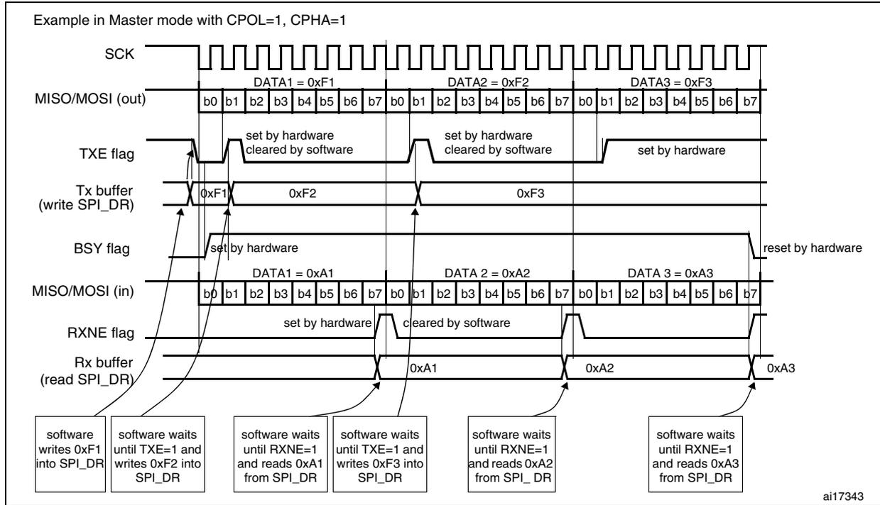
**Figure 200. TXE/RXNE/BSY behavior in Slave / full-duplex mode (BIDIMODE=0, RXONLY=0) in the case of continuous transfers**
