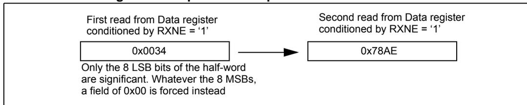
**Figure 223. LSB justified 16-bit extended to 32-bit packet frame with CPOL = 0**
