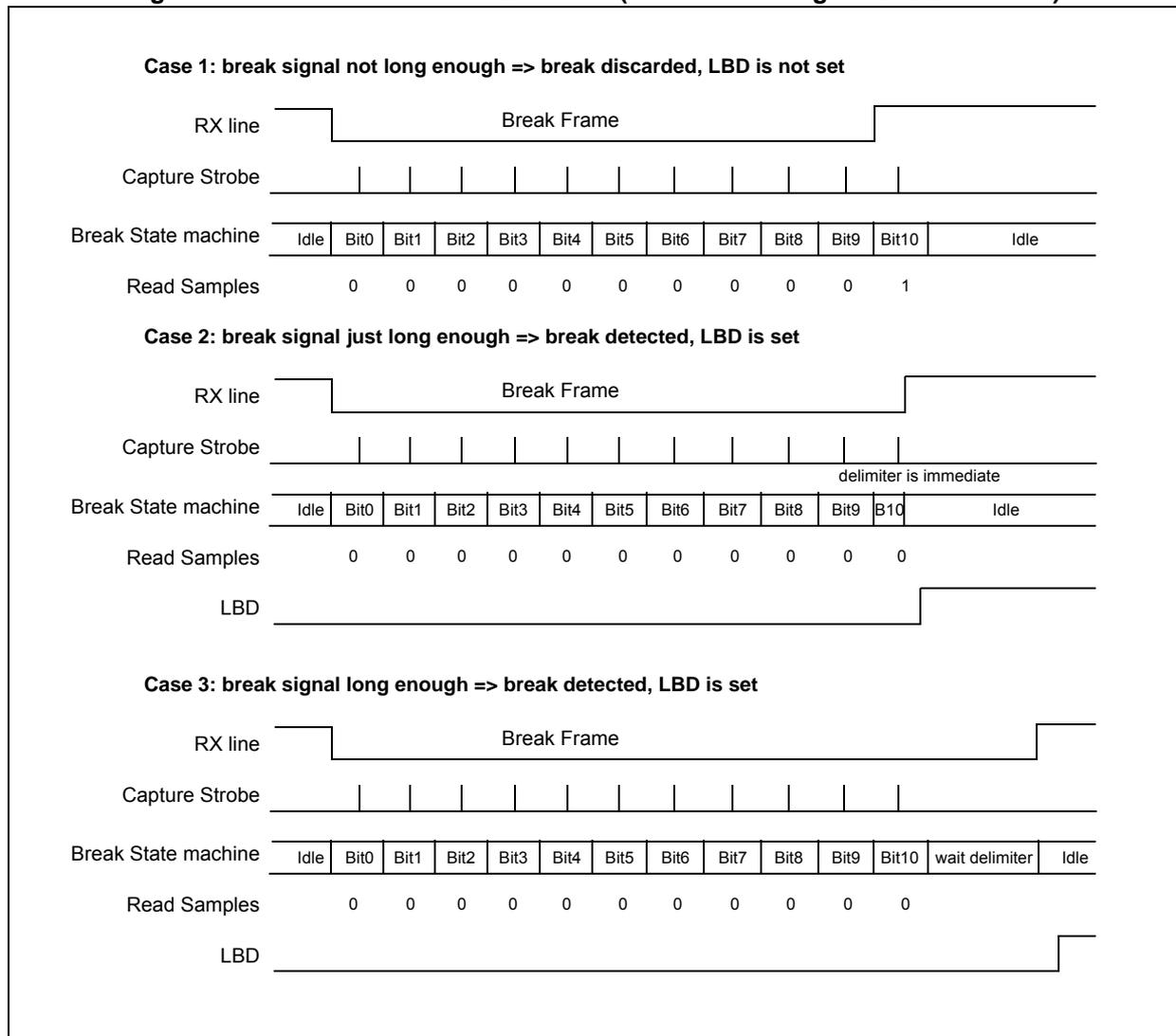
Figure 177. Break detection in LIN mode vs. Framing error detection
