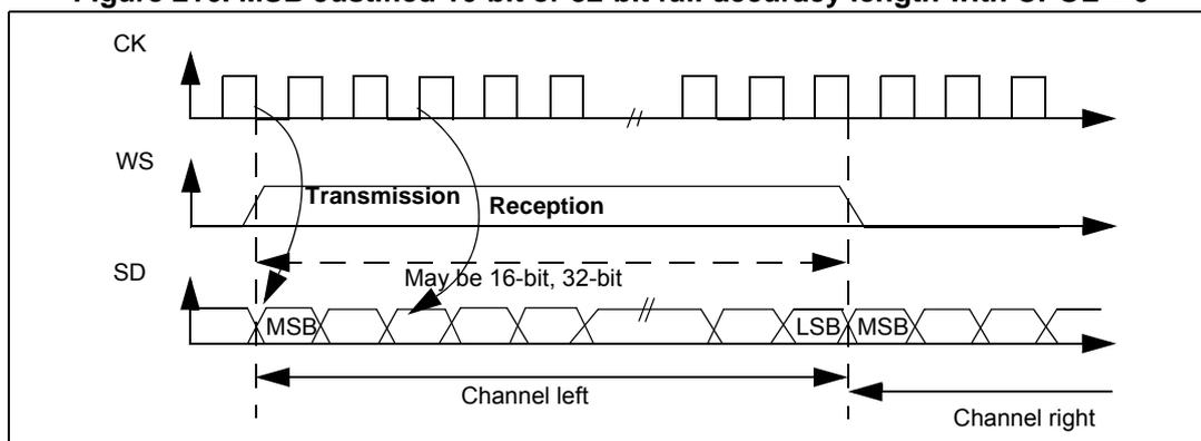
Data are latched on the falling edge of CK (for transmitter) and are read on the rising edge (for the receiver).
