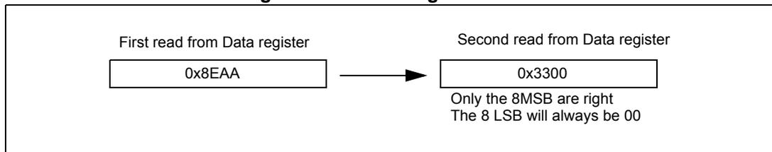
**Figure 214. I<sup>2</sup>S Philips standard (16-bit extended to 32-bit packet frame with CPOL = 0)**
