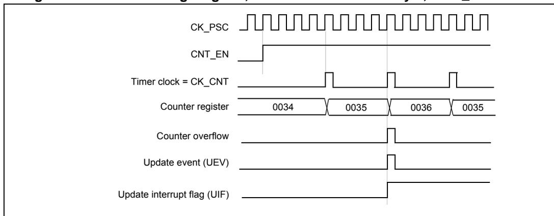
1. Center-aligned mode 2 or 3 is used with a UIF on overflow.
