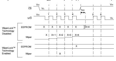
Microchip's non-volatile digital potentiometers adopt a methodology called WiperLock technology to ensure that once the non-volatile wiper is "locked" the wiper setting cannot be modified except with "high-voltage" commands. This inhibits accidental modification of the wiper setting during normal operation.
