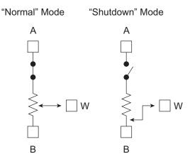
The software shutdown allows control to each of the resistor network terminal pins. Each resistor network has 4-bit in a TCON register. One bit for each terminal pin (A, B and W) and one bit that mimics the hardware shutdown state (the resistor network is disconnected from the Terminal A pin and the Wiper value is forced to 00h).
