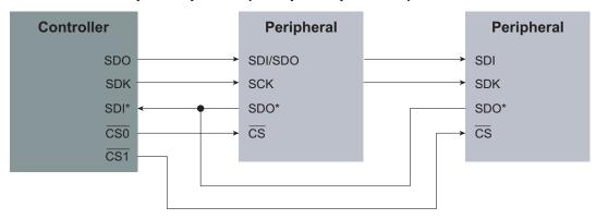
\*This connection is optional and only required for read operations. Additional circuitry may be required for ORing of the peripheral SDO signals based on the device selected.
