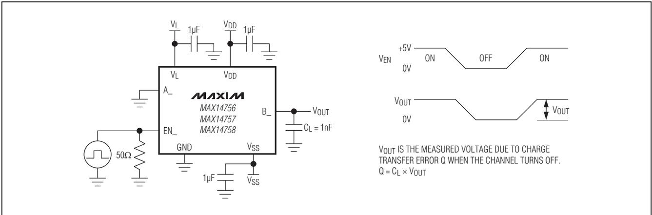
Figure 8. Charge Injection
