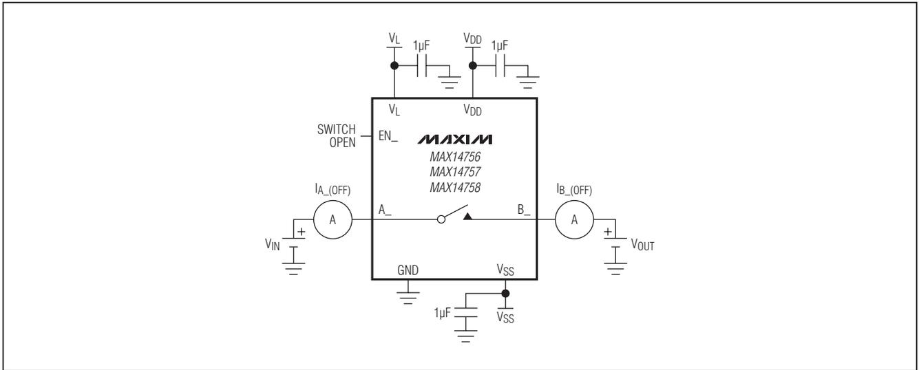
Figure 3. Off-Leakage Current
