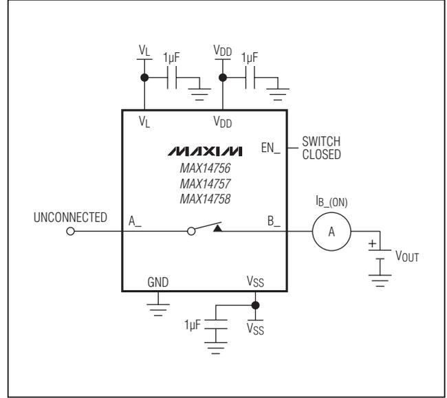
Figure 2. On-Leakage Current
