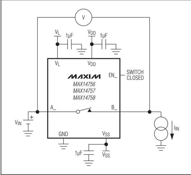
Figure 1. On-Resistance Measurement
