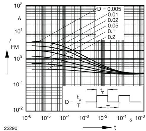
Fig. 2 - Peak forward current  $I_{FM} = f(t_p)$
