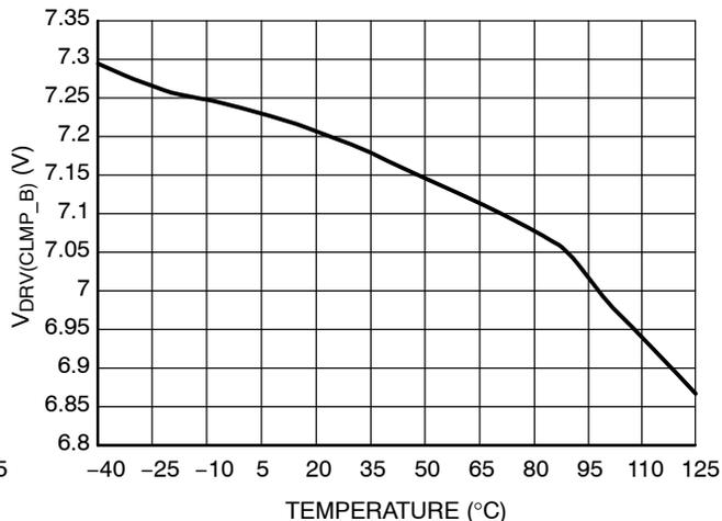
**Figure 17. Driver Clamp Level – B Version,
