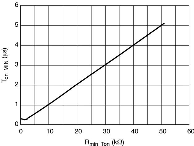
**Figure 49. Min T<sub>on</sub> Adjust Characteristic**
