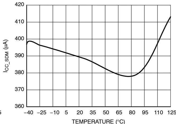
Figure 7. Startup Current
