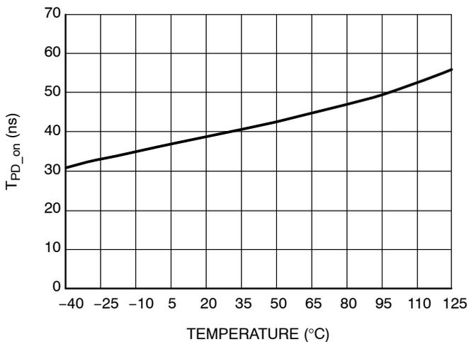
**Figure 18. CS to DRV Turn-on Propagation
