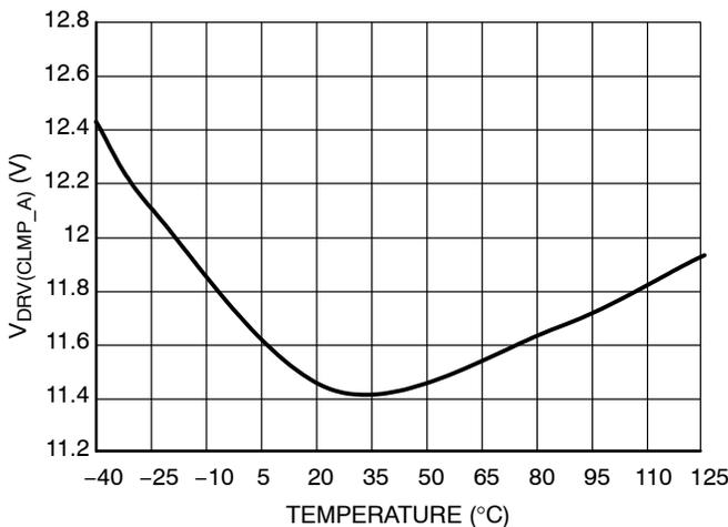
Figure 14. Driver Clamp Level – A Version,  $V_{CC} = 28\text{ V}$  and  $C_{load} = 1\text{ nF}$
