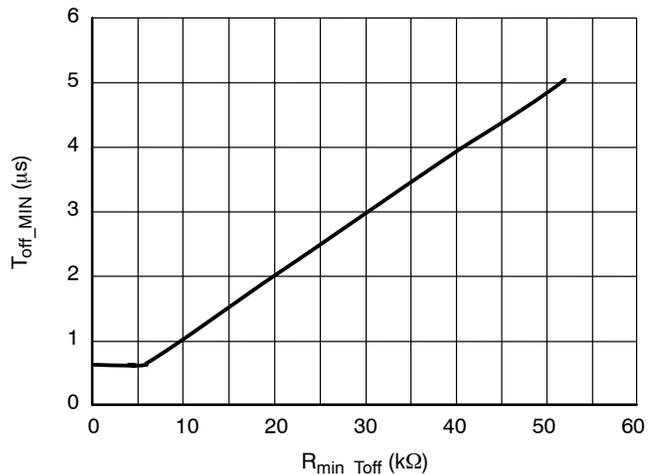
**Figure 50. Min T<sub>off</sub> Adjust Characteristic**
