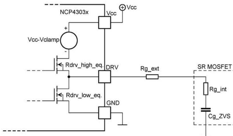
**Figure 54. Equivalent Schematic of Gate Drive Circuitry**
