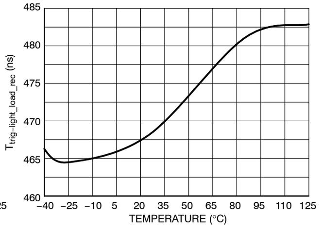
Figure 25. Light Load to Normal Operation Recovery Time
