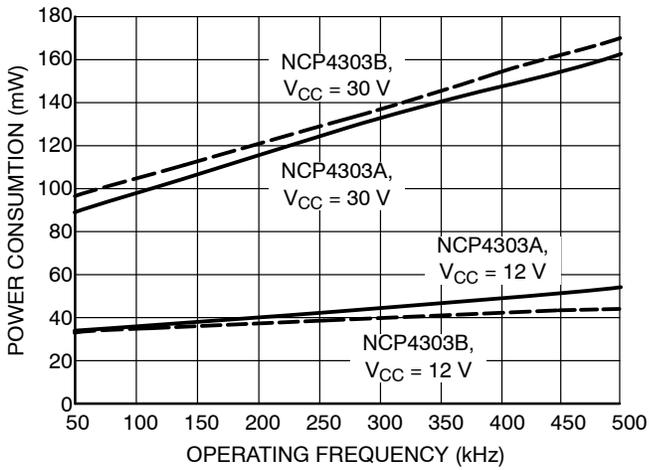
**Figure 55. IC Power Consumption as a Function of Frequency for  $C_{load} = 0$  nF,  $R_{ton\_min} = R_{toff\_min} = 5$  k $\Omega$**
