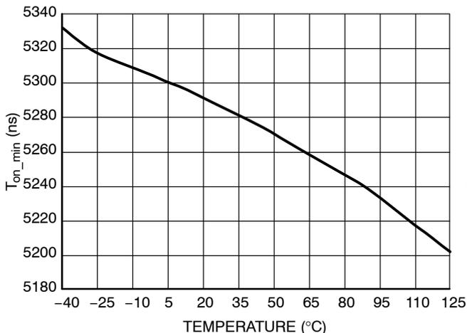
**Figure 30. Minimum on Time @  $R_{t\_on\_min} = 53\text{ k}\Omega$**
