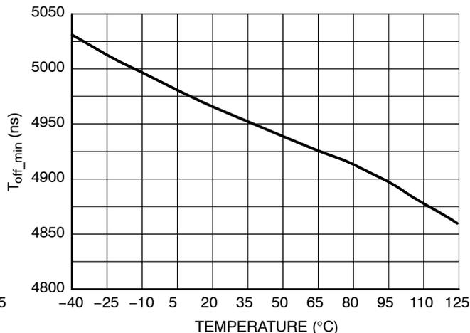
**Figure 31. Minimum Off Time @  $R_{t\_off\_min} = 53\text{ k}\Omega$**
