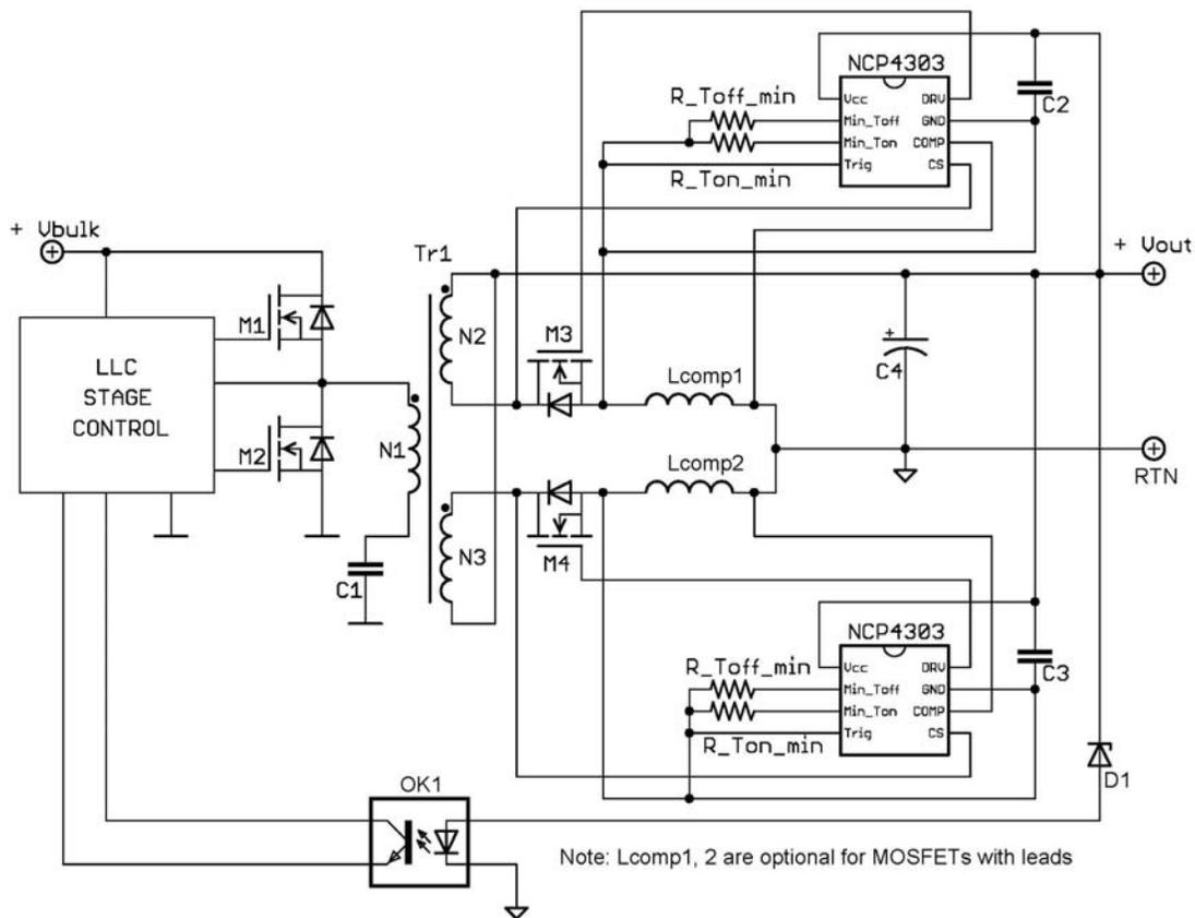
Figure 1. Typical Application Example – LLC Converter
