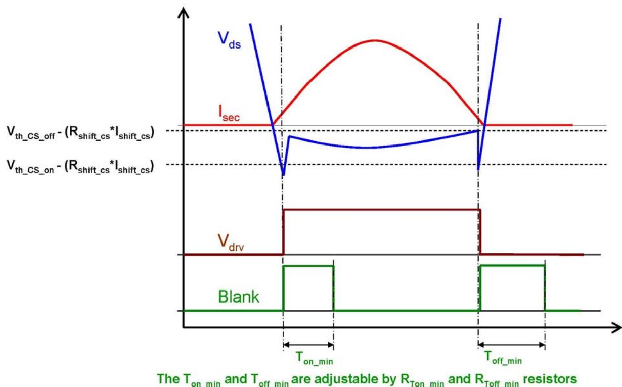
Figure 34. ZCD Comparators Thresholds and Blanking Periods Timing
