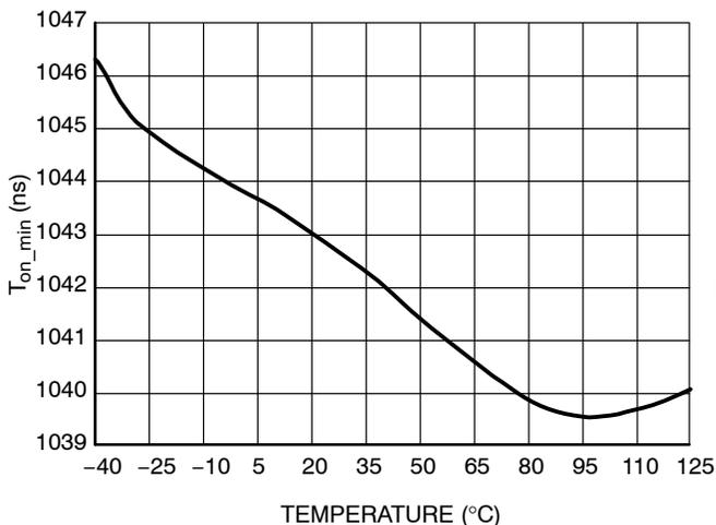
**Figure 28. Minimum on Time @  $R_{t\_on\_min} = 10\text{ k}\Omega$**
