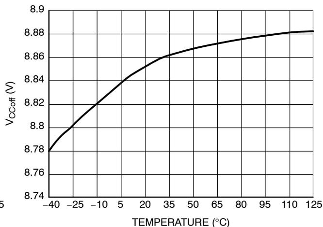
Figure 5. V<sub>CC</sub> Turn-off Voltage
