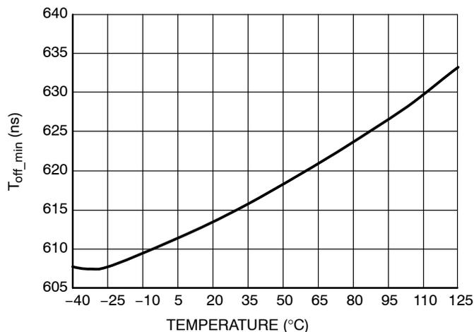
**Figure 32. Minimum Off Time @  $R_{t\_off\_min} = 0\ \Omega$**
