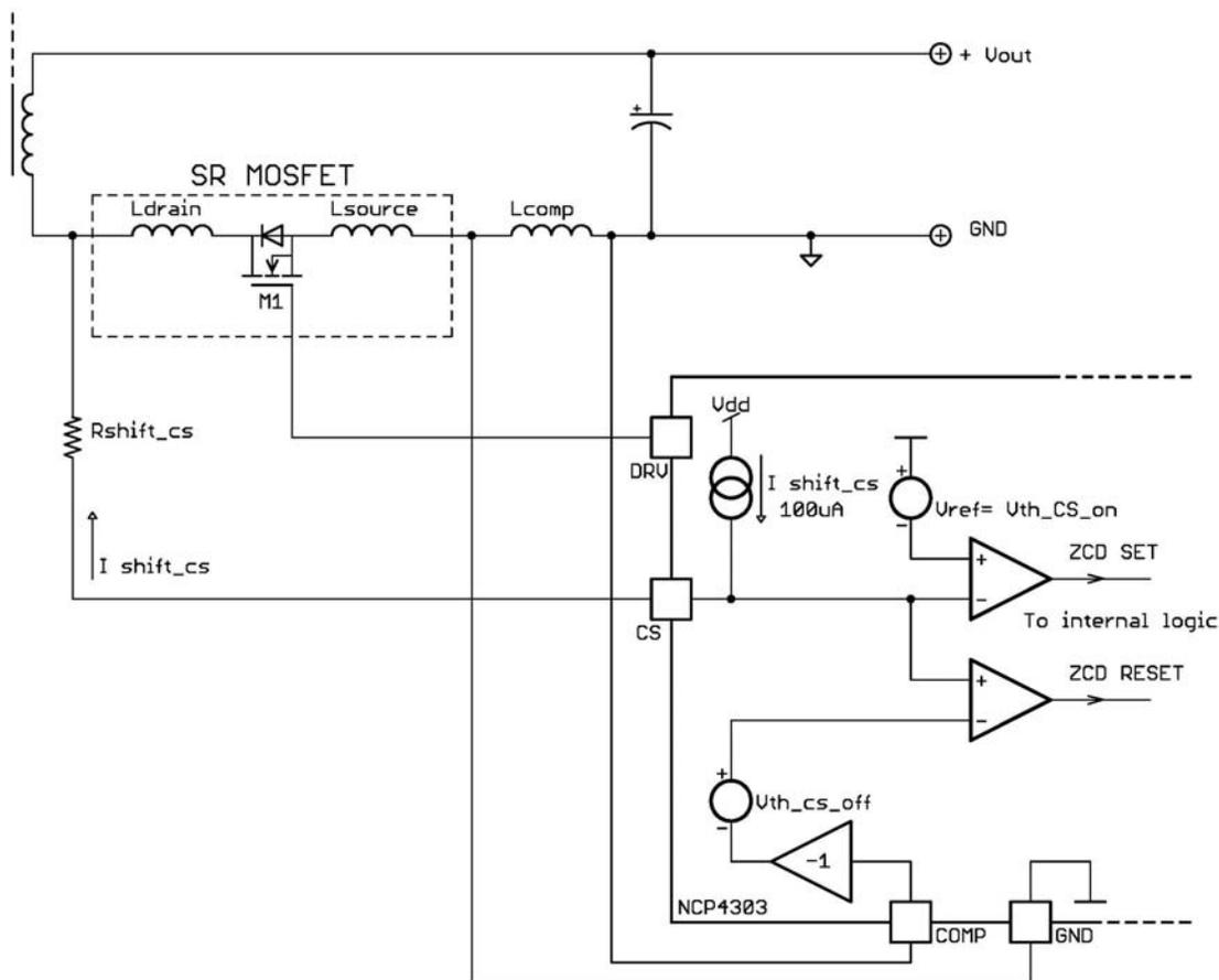
**Figure 33. ZCD Sensing Circuitry Functionality**
