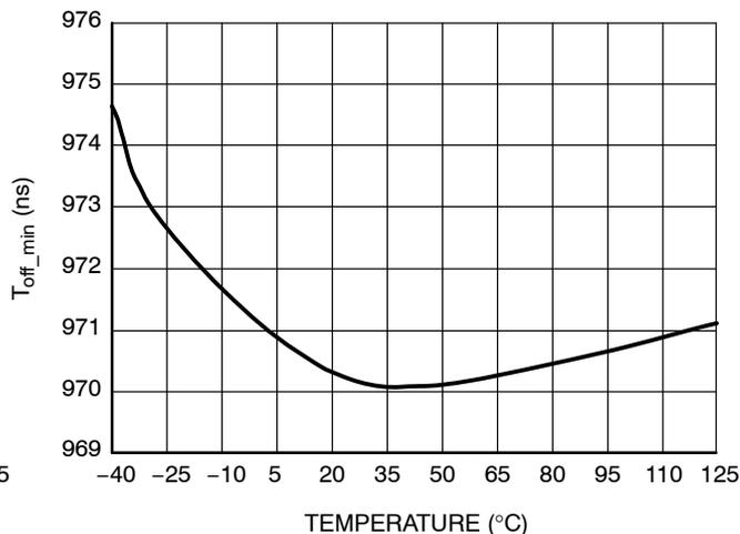
**Figure 29. Minimum Off Time @  $R_{t\_off\_min} = 10\text{ k}\Omega$**
