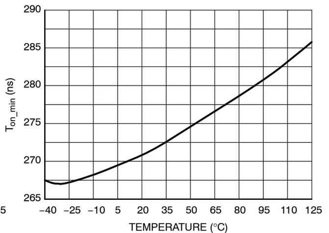
Figure 27. Minimum on Time @ R<sub>t\_on\_min</sub> = 0 Ω
