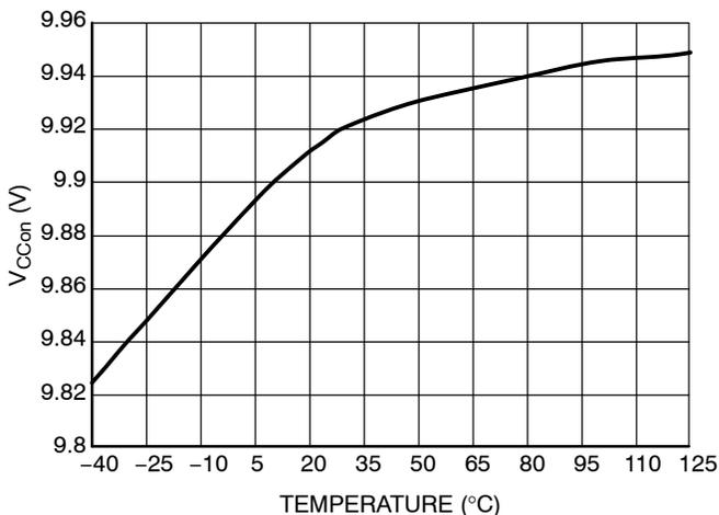
Figure 4. V<sub>CC</sub> Startup Voltage
