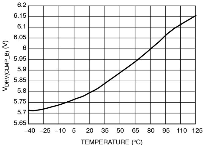
**Figure 16. Driver Clamp Level – B Version,
