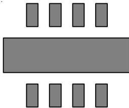
(c) Copper Area =  $30\text{mm}^2$ ,  $\theta_{JA} = 54^\circ\text{C/W}$
