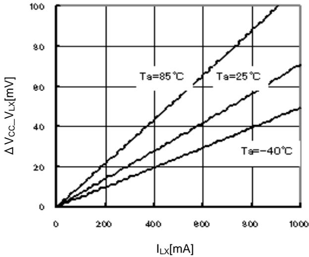
Figure 14. High Side FET ON-Resistance Temperature Characteristics
