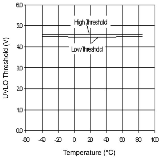
Figure 7. UVLO Threshold Voltage vs Temperature
