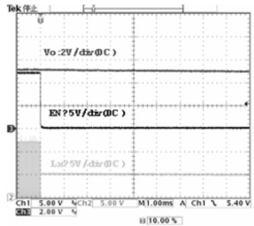
Figure 25. Stop Waveform
