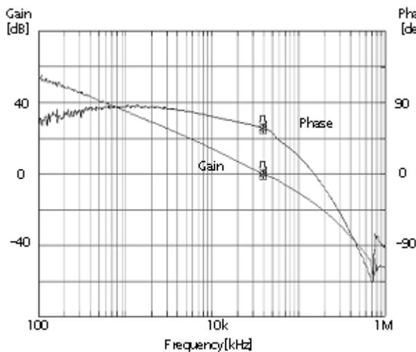
Figure 20. Frequency Response Characteristics (I<sub>o</sub>=1.5A)
