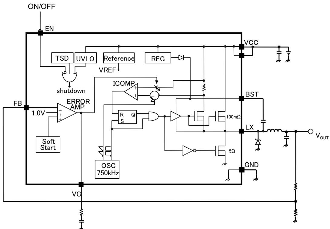
Figure 3. Block Diagram
