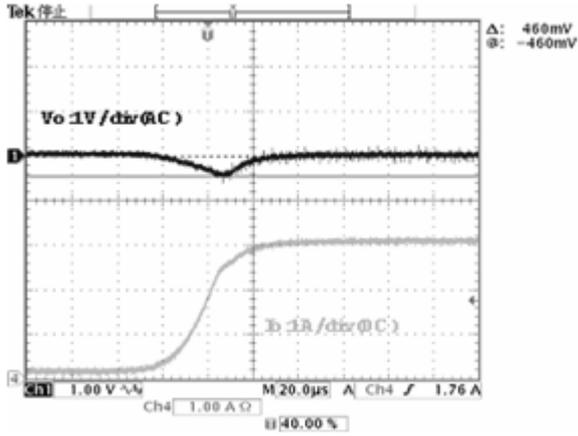
Figure 22. Load Response Characteristics (Io=0A to 3A)
