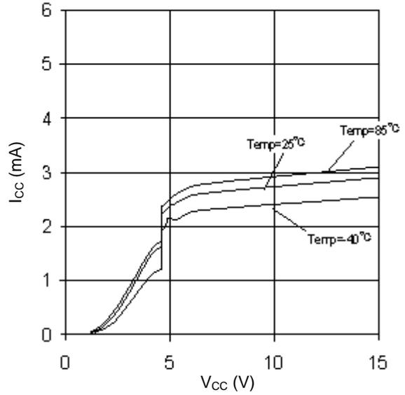
Figure 5. Circuit Current vs  $V_{CC}$
