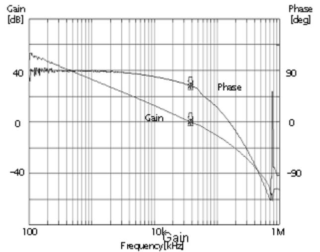
Figure 21. Frequency Response Characteristics (I<sub>o</sub>=3.0A)
