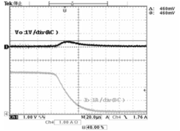
Figure 23. Load Response Characteristics (Io=3A to 0A)
