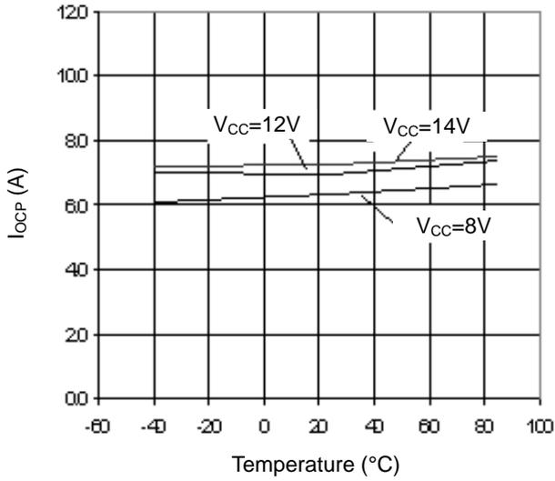
Figure 16. OCP Detect Current vs Temperature
