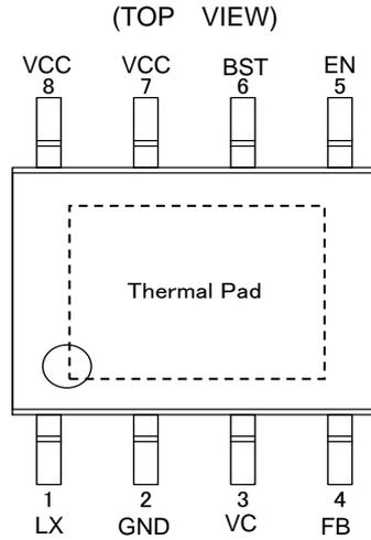
Figure 2. Pin Configuration
