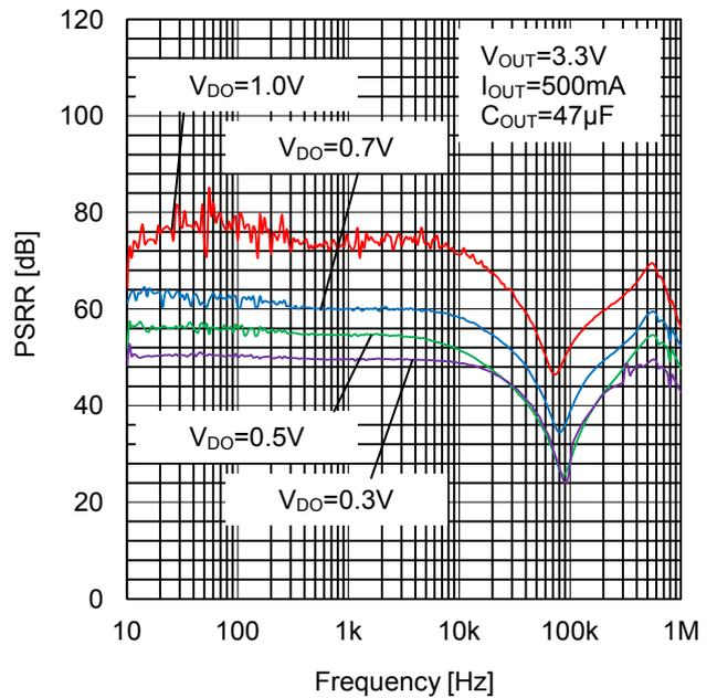
Figure 16. Power-Supply Rejection Ratio vs  $V_{DO}$
