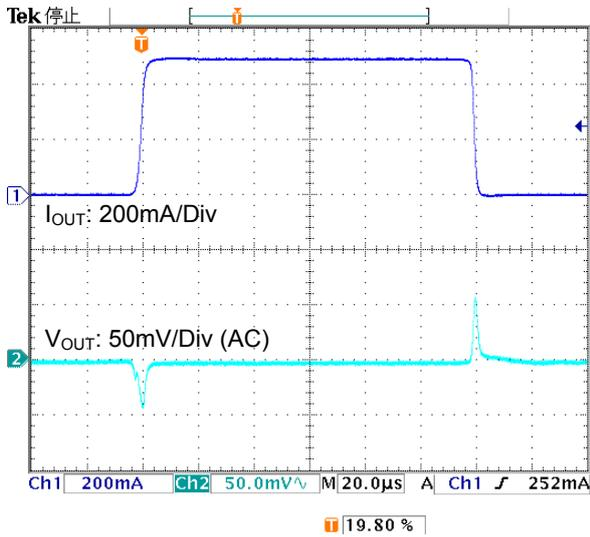
Figure 21. Load Transient
