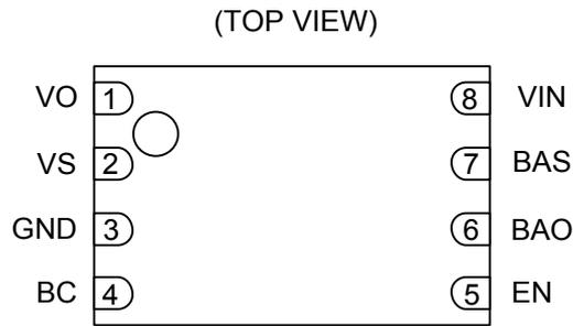
Figure 2. Pin Configuration
