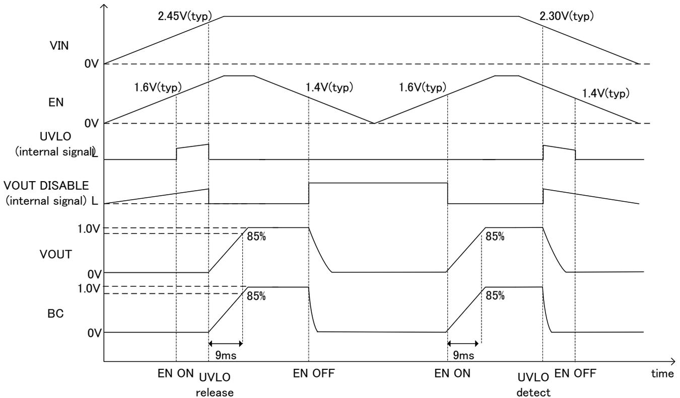
Figure 4. The Waveform During VIN/EN Rising and Falling
