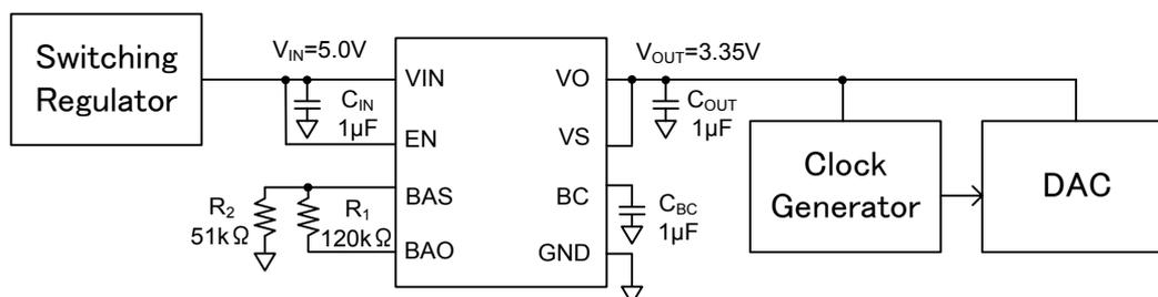
Figure 1. Basic Application Circuit Diagram (V<sub>OUT</sub>=3.35V)
