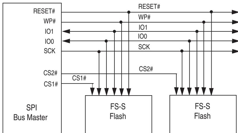
**Figure 2.3** Bus Master and Memory Devices on the SPI Bus — Quad Bit Data Path
