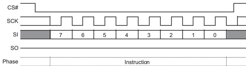
**Figure 9.53** Erase or Program Resume Command Sequence QPI Mode
