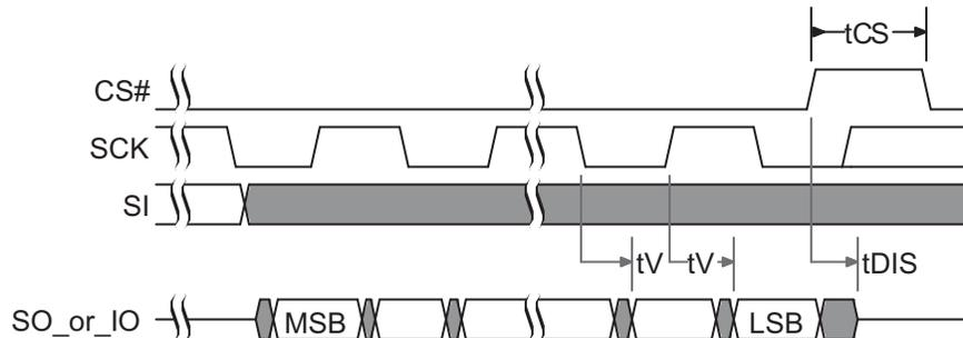
**Figure 5.16 SPI DDR Data Valid Window**
