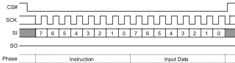
**Figure 3.5 Single Bit Wide Output Command**
