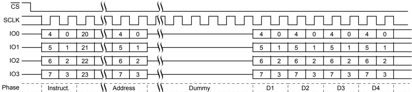
**Figure 9.21** ECCRD (19h), QPI Mode, CR2[7] = 1, or 4ECCRD (18h) Command Sequence
