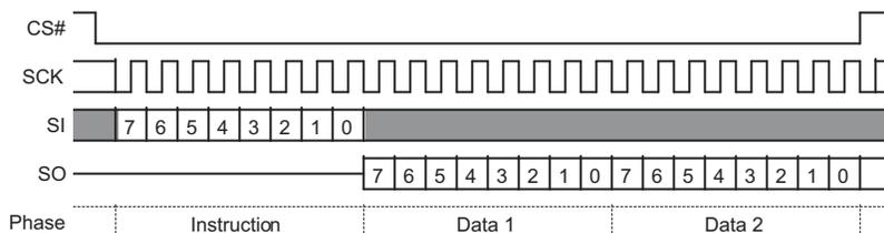
**Figure 3.6** Single Bit Wide I/O Command without latency
