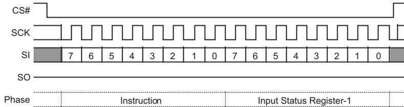
**Figure 9.11** Write Registers (WRR) Command Sequence – 16 Data Bits
