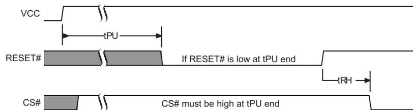
**Figure 5.5** Reset High at the end of POR
