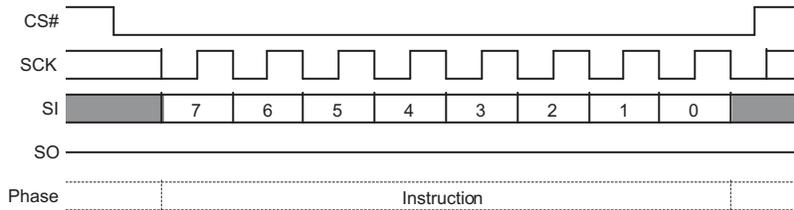
**Figure 3.4 Single Bit Wide Input Command**
