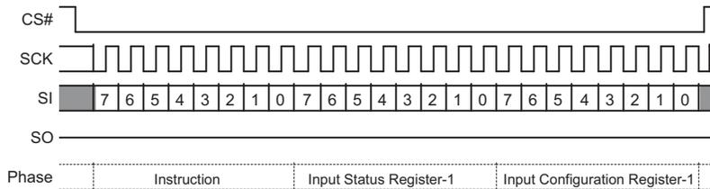
**Figure 9.12** Write Registers (WRR) Command Sequence – 16 Data Bits QPI Mode
