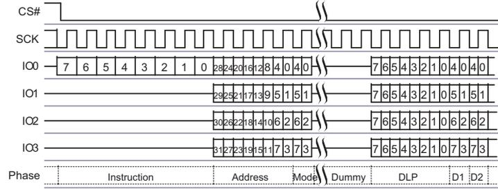
Figure 3.12 DDR Quad I/O Read in QPI Mode
