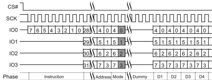
**Figure 3.10** Quad I/O Read Command in QPI Mode
