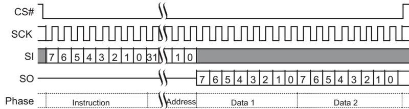
**Figure 3.7** Single Bit Wide I/O Command with latency
