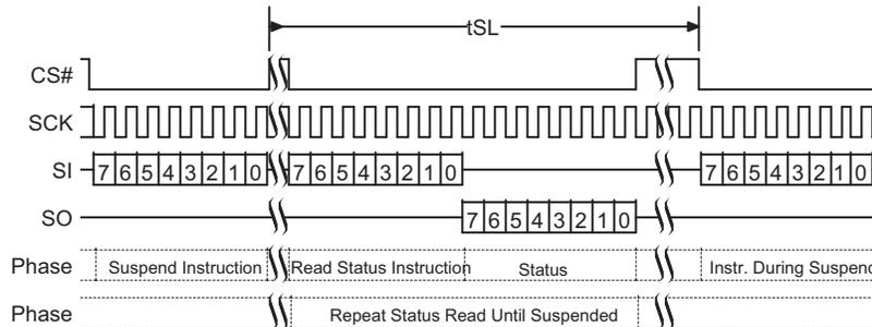
**Figure 9.50** Erase or Program Suspend Command Sequence
