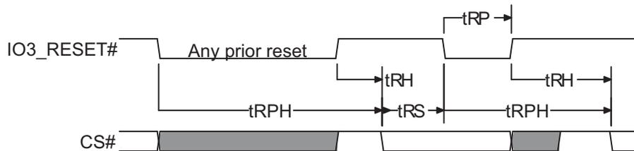
**Figure 5.8 Hardware Reset when Quad Mode and IO3 / Reset# are Enabled**
