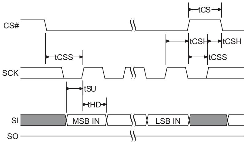
**Figure 5.11 SPI Single Bit Output Timing**
