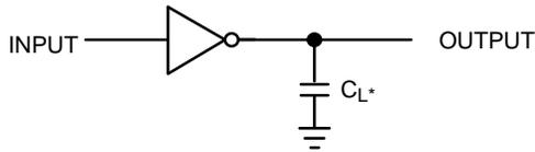
\*Includes all probe and jig capacitance.
