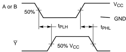
**Figure 3. Switching Waveforms**
