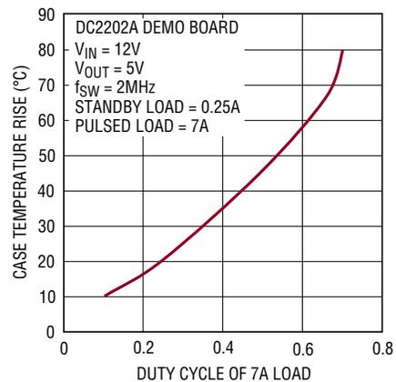
Figure 7. Case Temperature Rise vs 7A Pulsed Load
