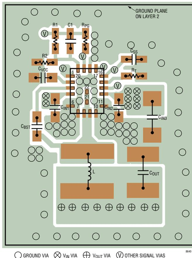
Figure 1. Recommended PCB Layout for the LT8640/LT8640-1
