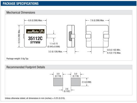
Specifications typical at  $T_{\rm A} = 25^{\circ}{\rm C}$
