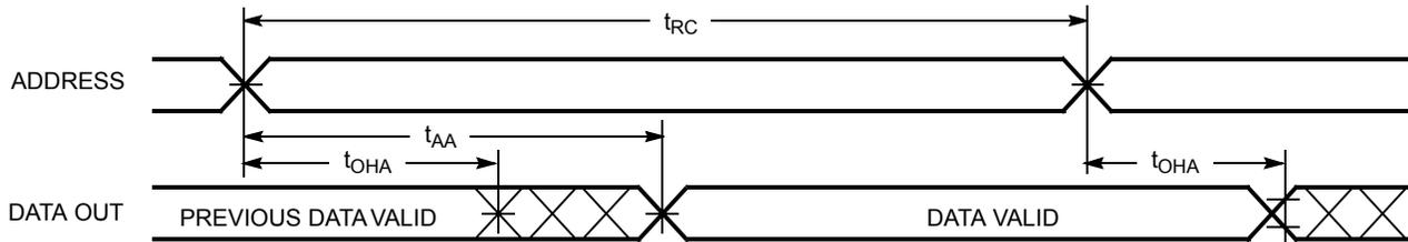
**Figure 5. Read Cycle No. 2 (Either Port  $\overline{CE}/\overline{OE}$  Access)** [21, 24, 25]
