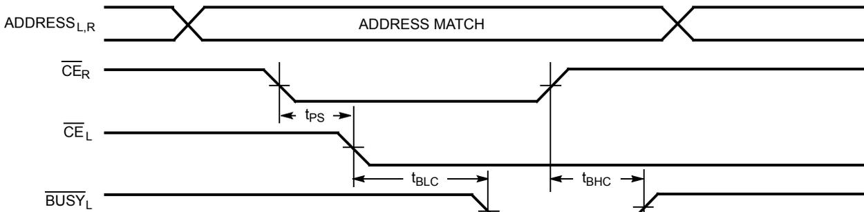
Figure 14. Busy Timing Diagram No. 2 (Address Arbitration) [40]
