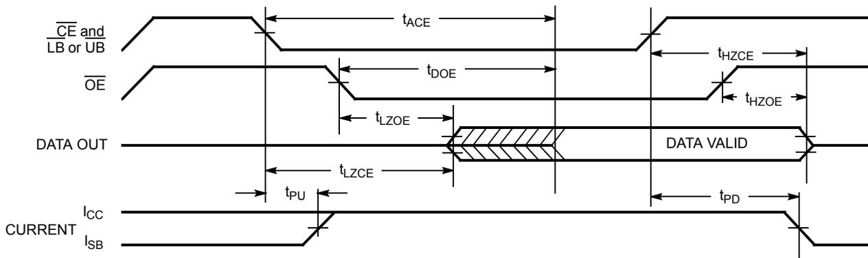
**Figure 6. Read Cycle No. 3 (Either Port)** [21, 23, 24, 25]
