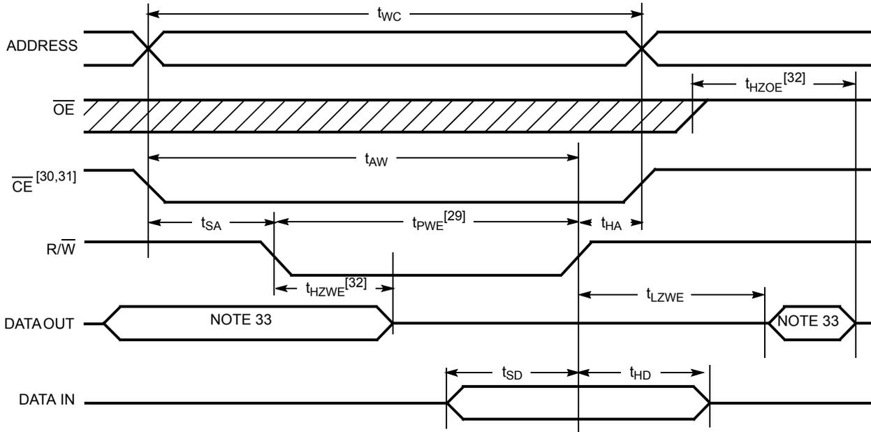
Figure 8. Write Cycle No. 2: CE Controlled Timing [26, 27, 28, 34]
