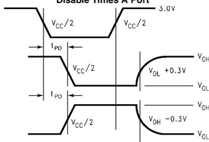
**Voltage Waveforms Propagation Delay and Setup and Hold Times**
