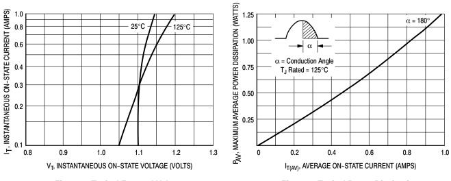
Figure 3. Typical Forward Voltage
