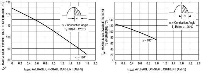
Figure 1. Maximum Case Temperature
