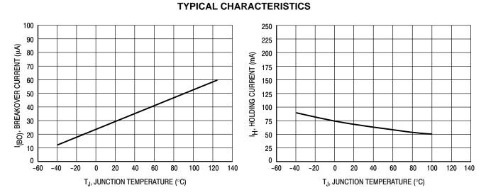
Figure 6. Typical Breakover Current
