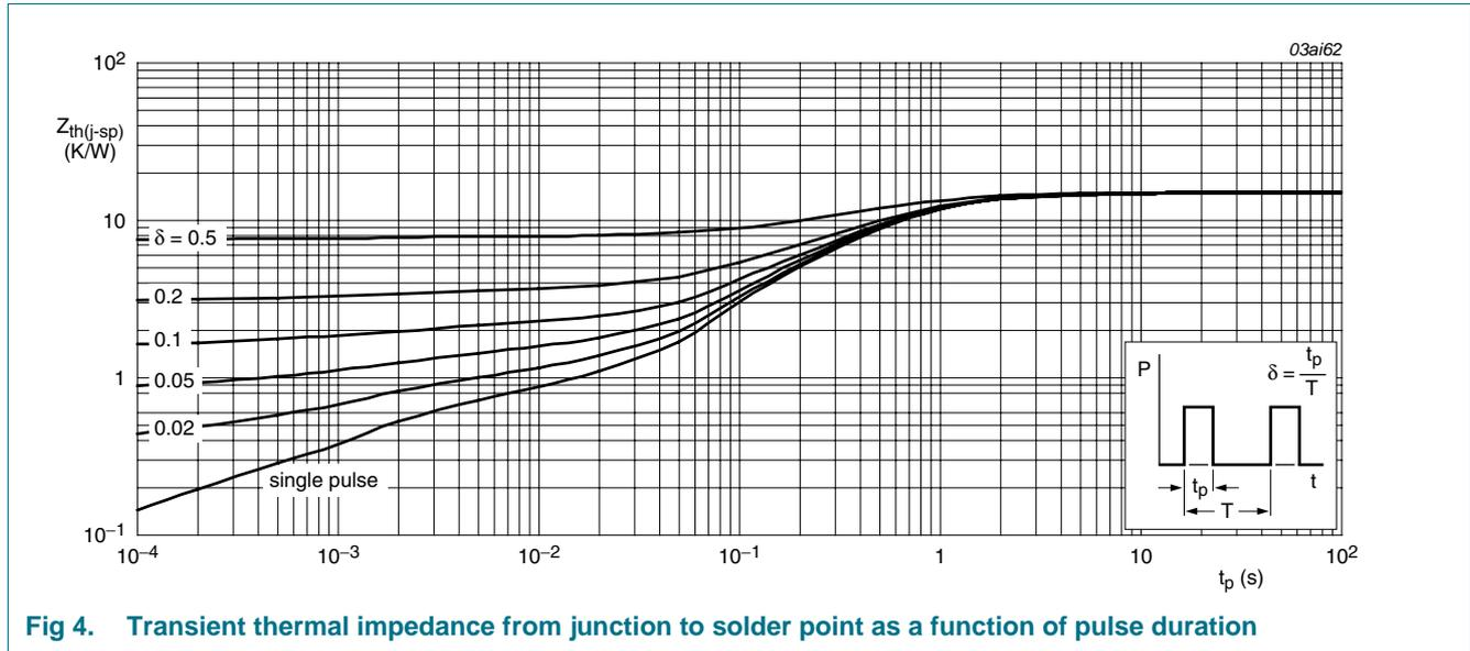
**Fig 4. Transient thermal impedance from junction to solder point as a function of pulse duration**
