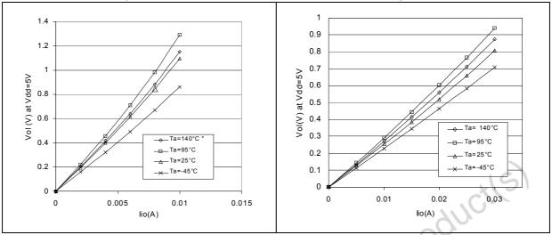
Figure 83. Typical  $V_{OH}$  at  $V_{DD} = 5V$
