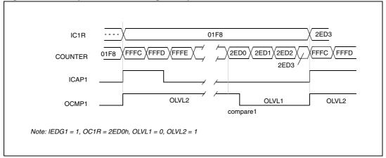
Figure 53. Pulse width modulation mode timing example with 2 output compare functions
