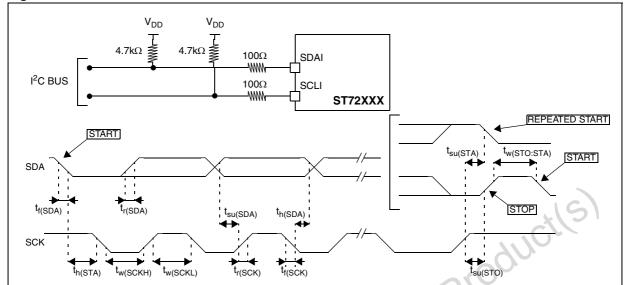
Figure 93. Typical application with I<sup>2</sup>C BUS and timing diagram<sup>(1)</sup>
