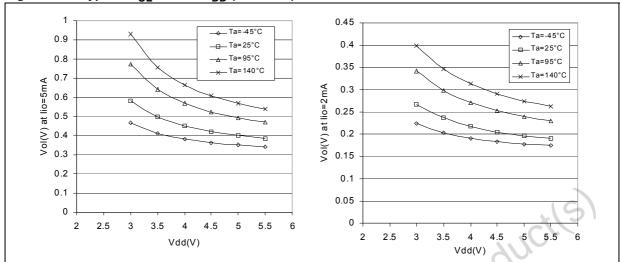
Figure 85. Typical V<sub>OL</sub> versus V<sub>DD</sub> (high-sink)
