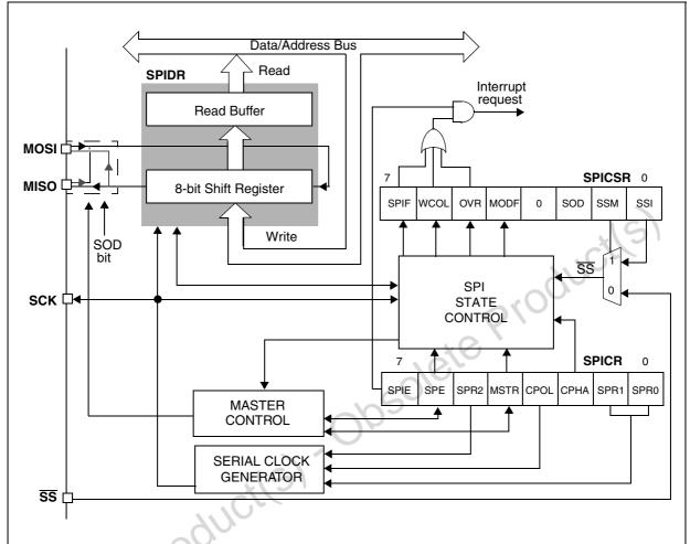
Figure 55. Serial peripheral interface block diagram
