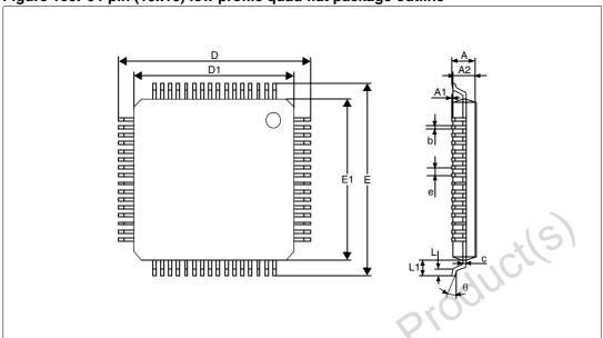
Figure 100. 64-pin (10x10) low profile quad flat package outline
