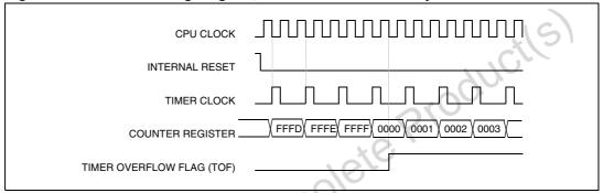
Figure 44. Counter timing diagram, internal clock divided by 4
