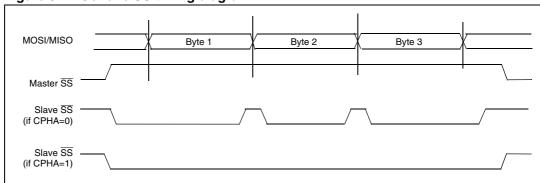
Figure 57. Generic SS timing diagram
