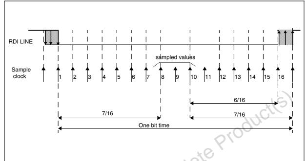
Figure 65. Bit sampling in reception mode
