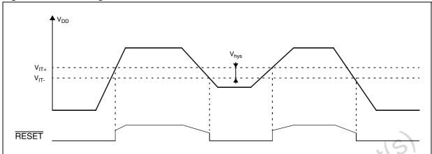
Figure 14. Low voltage detector versus reset
