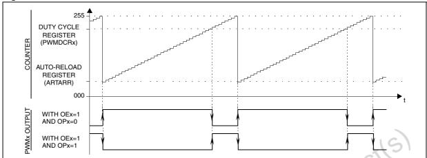
Figure 37. PWM auto-reload timer function
