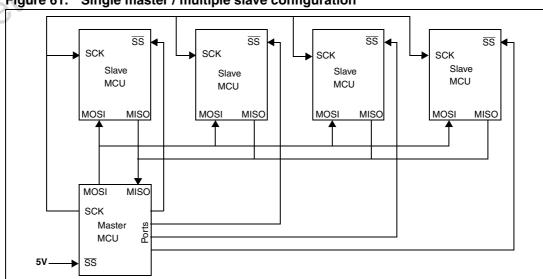
Figure 61. Single master / multiple slave configuration
