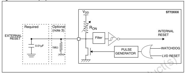
Figure 87. RESET pin protection when LVD is enabled
