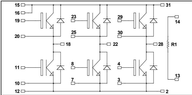
It is recommended to connect a decoupling capacitor between pins 31 & 2 to reduce switching overvoltages, if DC Power is connected between pins 15, 16 & 12. Pins 15 & 16 must be shorted together.
