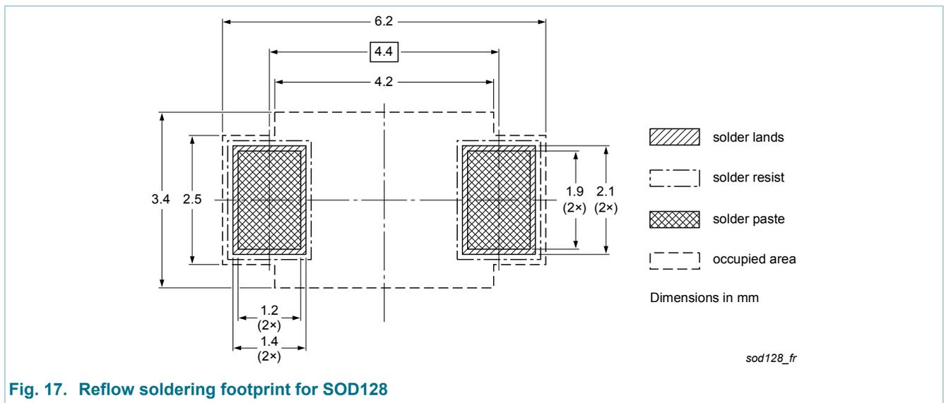
Fig. 17. Reflow soldering footprint for SOD128
