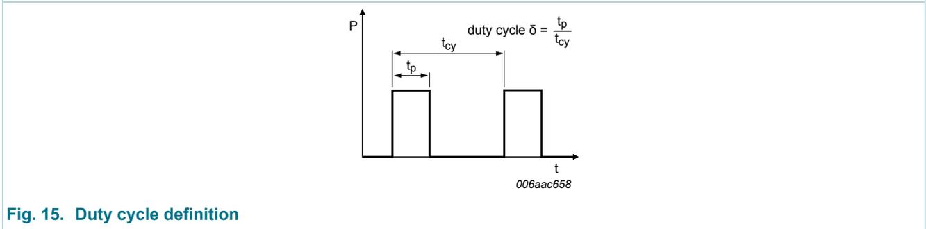
Fig. 15. Duty cycle definition
