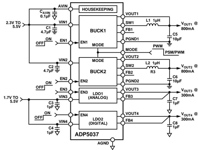
Figure 52. ADP5037 Fixed Output Voltages with Enable Pins
