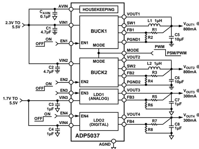
Figure 50. Processor System Power Management with PSM/PWM Control
