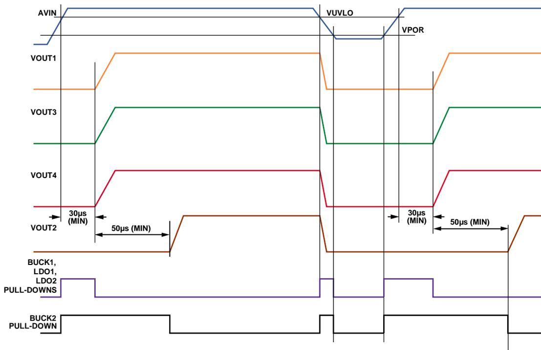
Figure 46. Regulator Sequencing on the ADP5037 (EN1 = EN2 = EN3 = EN4 = V<sub>AVIN</sub>)
