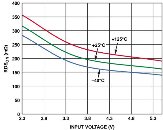
Figure 32. NMOS  $R_{DS(on)}$  vs. Input Voltage Across Temperature
