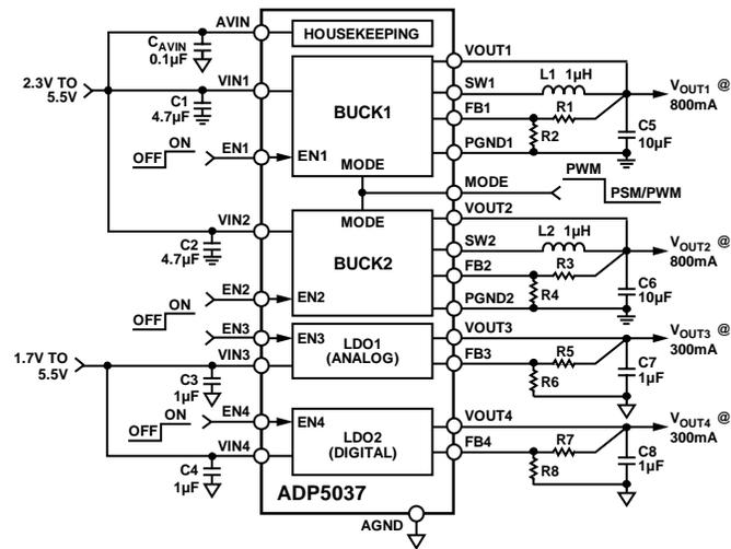
Figure 53. ADP5037 Adjustable Output Voltages with Enable Pins
