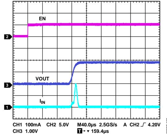
Figure 30. LDO Startup,  $V_{OUT3} = 1.8$  V
