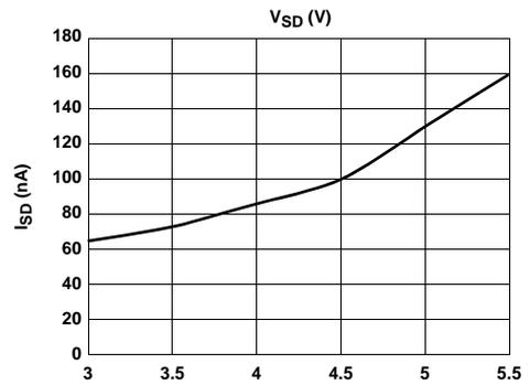
FIGURE 2. DIGITAL SUPPLY CURRENT vs DIGITAL SUPPLY VOLTAGE
