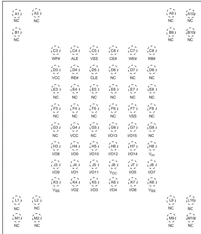
**Figure 1.5** 67-BGA Contact (Balls Down, Top View) (S34MS01G2, S34MS02G2)
