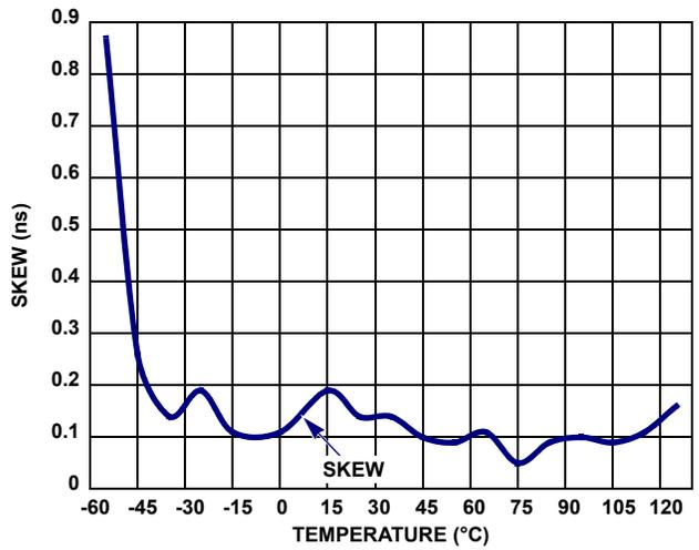
FIGURE 13. DRIVER DIFFERENTIAL SKEW vs TEMPERATURE (ISL3158AE)
