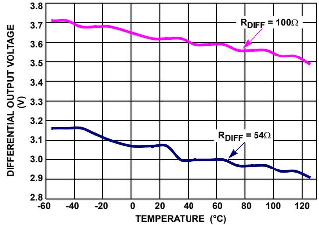
FIGURE 9. DRIVER DIFFERENTIAL OUTPUT VOLTAGE vs TEMPERATURE
