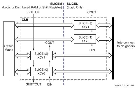
Figure 5-1: Arrangement of Slices within the CLB
