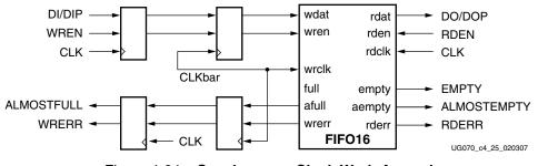
Figure 4-24: Synchronous Clock Work-Around
