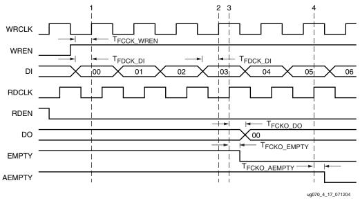
Figure 4-17: Writing to an Empty FIFO in FWFT Mode
