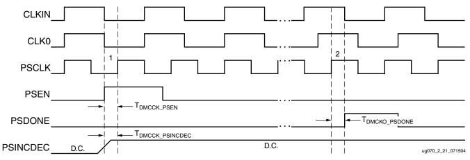
Figure 2-22: Phase Shift Example: Variable
