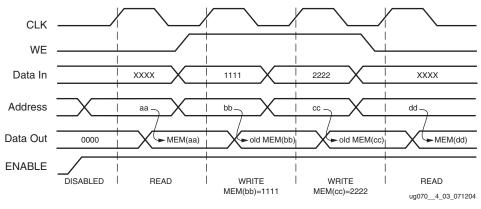
Figure 4-3: **READ\_FIRST Mode Waveforms**
