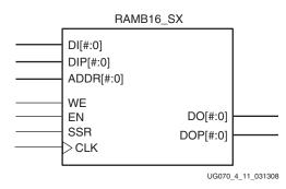
Figure 4-11: Single-Port Block RAM Primitive
