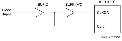
Figure 8-7: Clocking Arrangement Using BUFIO and BUFR
