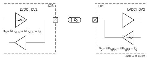
Figure 6-32: Controlled Impedance Driver with Half Impedance Bidirectional Termination
