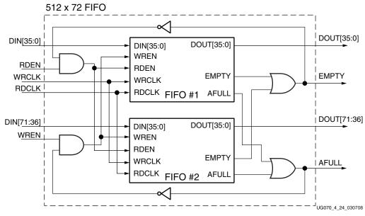
Figure 4-23: Cascading FIFO by Width
