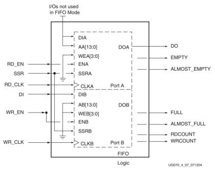
Figure 4-7: Block RAM Implemented as a FIFO
