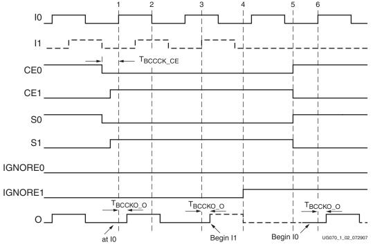
The timing diagram in Figure 1-2 illustrates various clock switching conditions using the BUFGCTRL primitives. Exact timing numbers are best found using the speed specification.
