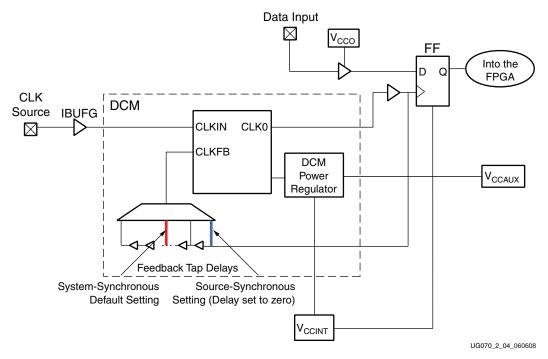
Figure 2-4: DCM and Feedback Tap-Delay Elements
