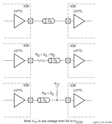
Figure 6-25: LVTTL Unidirectional Termination
