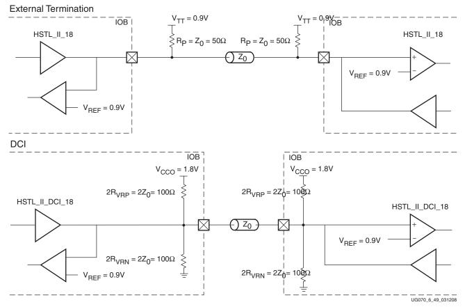
Figure 6-51: HSTL Class II (1.8V) with Bidirectional Termination
