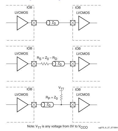
Figure 6-27: LVCMOS Unidirectional Termination
