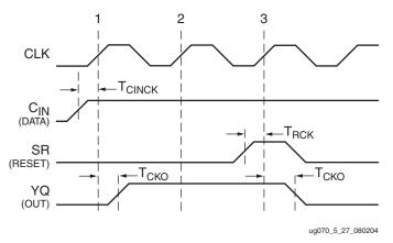
Figure 5-27: Slice Carry-Chain Timing Characteristics
