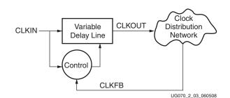
Figure 2-3: Simplified DLL Circuit
