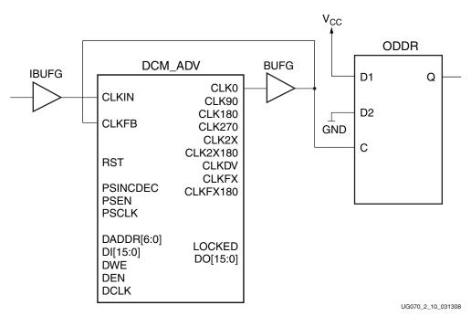
Figure 2-11: Board-Level Clock with Internal Feedback (Clock Forwarding)
