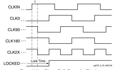
Figure 2-21: Phase Shift Example: Fixed
