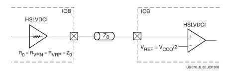
Figure 6-33: HSLVDCI Controlled Impedance Driver with Unidirectional Termination
