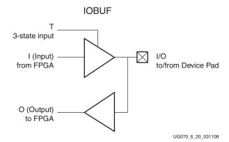
Figure 6-20: Input/Output Buffer (IOBUF) Primitive
