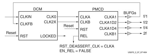
Figure 3-7: DCM and a Single PMCD
