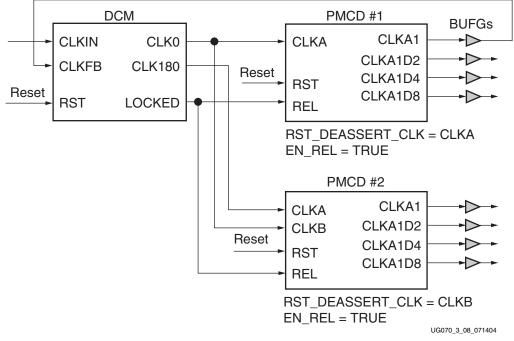
Figure 3-8: DCM and Parallel PMCDs
