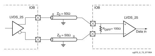
Figure 6-75: LVDS\_25 With DIFF\_TERM Receiver Termination
