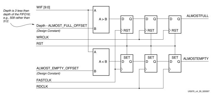
Figure 4-28: ALMOSTFULL and ALMOSTEMPTY Signal Generation
