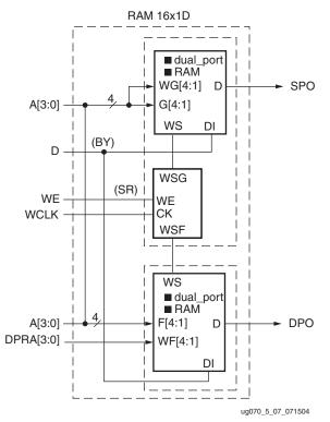
Figure 5-7: Dual-Port Distributed RAM (RAM16x1D)
