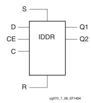
*Figure 7-8:* **IDDR Primitive Block Diagram**
