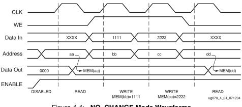
Figure 4-4: NO\_CHANGE Mode Waveforms
