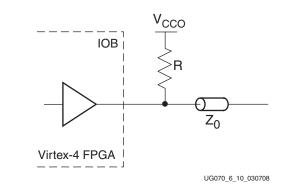
Figure 6-10: Driver with Termination to V<sub>CCO</sub> without DCI
