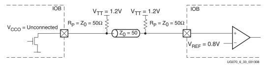
Figure 6-35: GTL with External Parallel Termination and Unconnected V<sub>CCO</sub>
