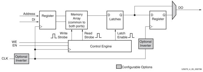
Figure 4-5: Block RAM Logic Diagram (One Port Shown)
