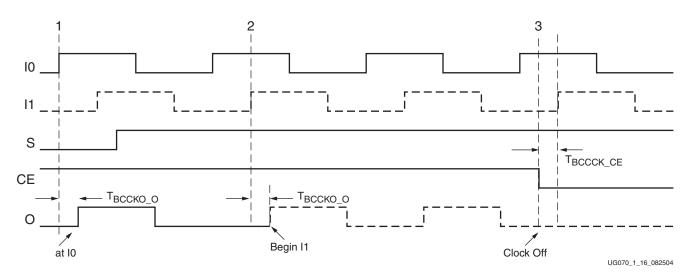
*Figure 1-16:* **BUFGMUX\_VIRTEX4 with a CE Timing Diagram**
