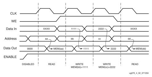
Figure 4-2: WRITE\_FIRST Mode Waveforms
