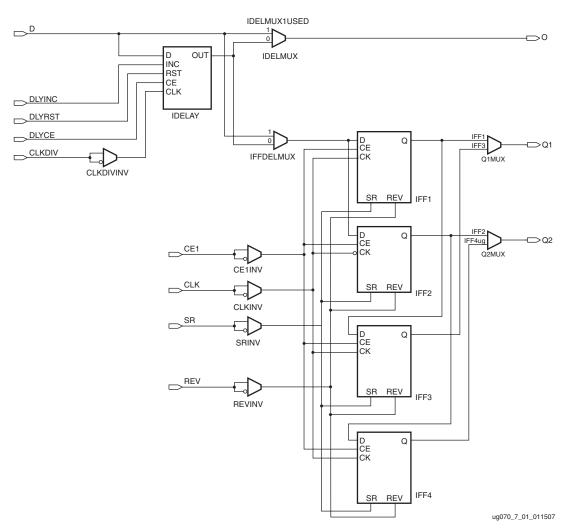
Figure 7-1: ILOGIC Block Diagram
