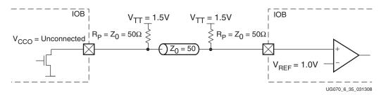
Figure 6-37: GTL+ with External Parallel Termination and Unconnected V<sub>CCO</sub>
