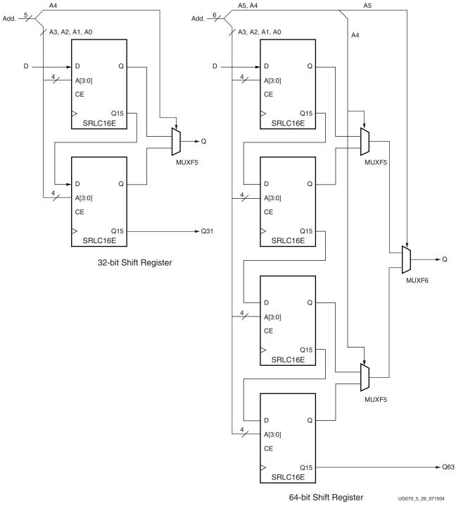
*Figure 5-29:* Shift-Register Submodules (32-bit, 64-bit)
