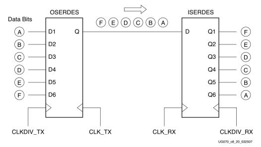
*Figure 8-3:* **Bit Ordering at Q1–Q6 Outputs of ISERDES**
