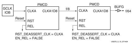
Figure 3-12: PMCD to PMCD for Clock Frequency Division
