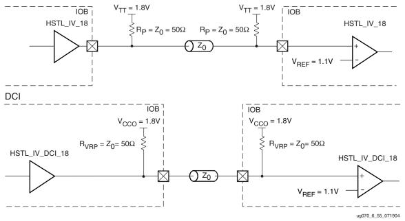
Figure 6-57: HSTL Class IV (1.8V) with Unidirectional Termination
