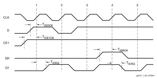
*Figure 7-9:* **ILOGIC Input Register Timing Characteristics**
