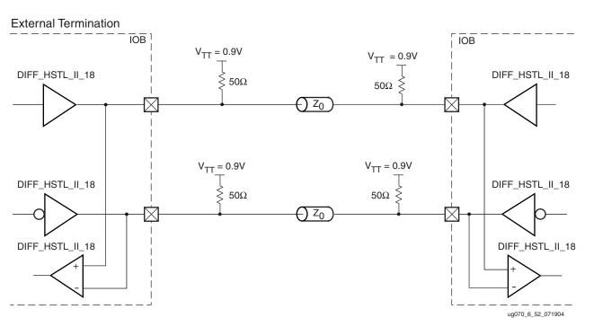
Figure 6-54 shows a sample circuit illustrating a valid termination technique for differential HSTL Class II (1.8V) with bidirectional termination.
