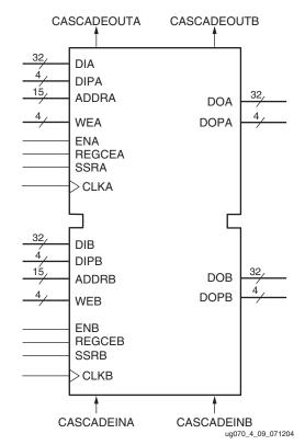
Figure 4-9: Block RAM Port Signals (RAMB16)
