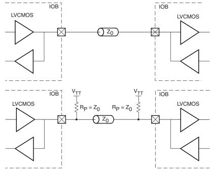
Note:  $V_{TT}$  is any voltage from 0V to  $V_{CCO}$
