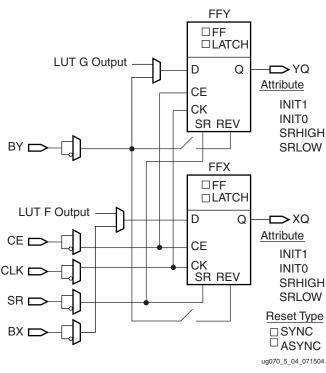
Figure 5-4: Register/Latch Configuration in a Slice
