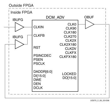
Figure 2-10: Board-Level Clock Using OBUF with External Feedback
