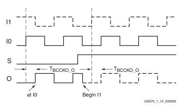
*Figure 1-14:* Asynchronous Mux Timing Diagram
