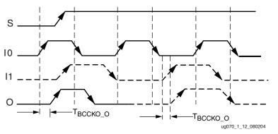
Figure 1-12: BUFGMUX\_VIRTEX4 Timing Diagram
