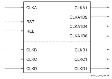
Figure 3-2: PMCD Primitive
