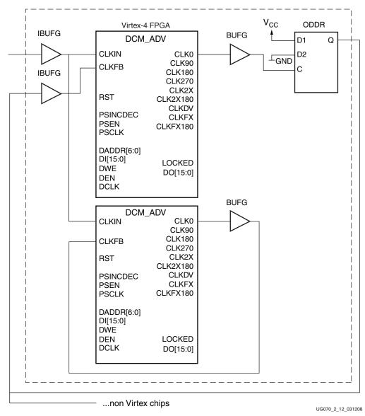
The example in Figure 2-13 shows an interface from Virtex-4 FPGAs to non-Virtex devices.
