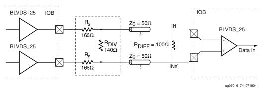
Figure 6-76: BLVDS Transmitter Termination
