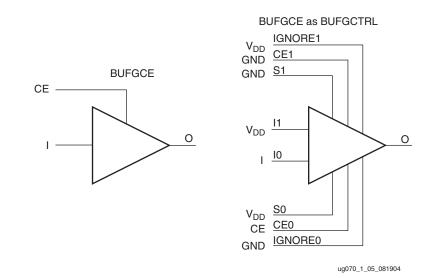
or Low. Figure 1-5 illustrates the relationship of BUFGCE and BUFGCTRL. A LOC constraint is available for BUFGCE and BUFGCE\_1.
