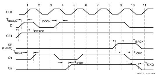
Figure 7-10: ILOGIC in IDDR Mode Timing Characteristics (OPPOSITE\_EDGE Mode)
