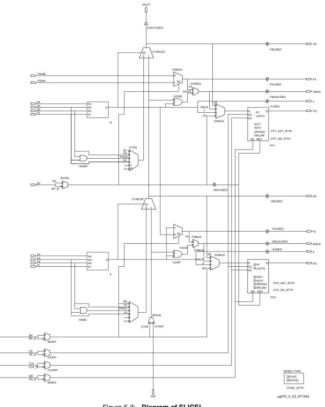
Figure 5-3: Diagram of SLICEL
