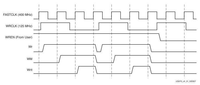
*Figure 4-30:* Write Timing Diagram
