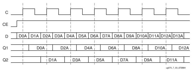
Figure 7-3: Input DDR Timing in OPPOSITE\_EDGE Mode
