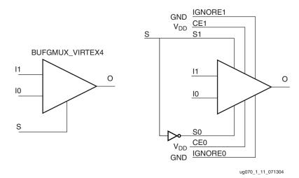
Figure 1-11: BUFGMUX\_VIRTEX4 as BUFGCTRL
