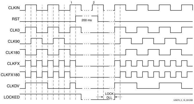
Figure 2-20: RESET/LOCK Example
