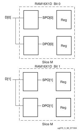
*Figure 5-8:* **Two RAM16X1D Placement**
