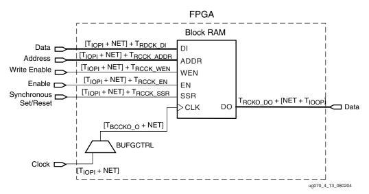
Figure 4-13: Block RAM Timing Model
