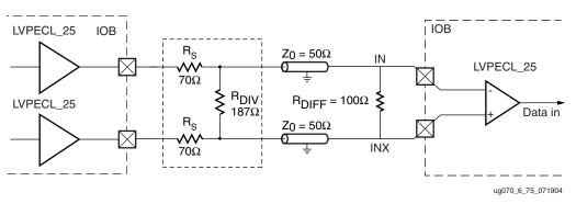
Figure 6-77: LVPECL Transmitter Termination
