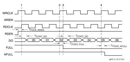
Figure 4-19: Reading From a Full FIFO
