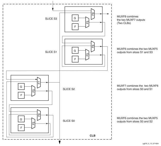
Figure 5-13: MUXF5 and MUXFX Multiplexers
