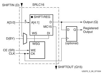
Figure 5-9: Shift Register Configurations
