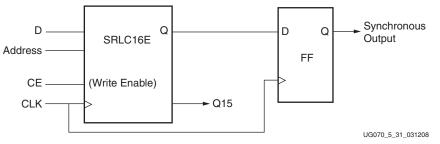
Figure 5-31: Fully Synchronous Shift Register
