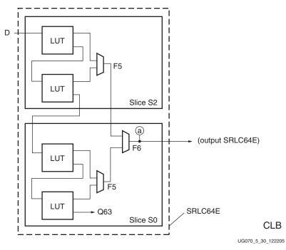
Figure 5-30: Shift Register Placement
