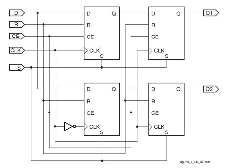
Figure 7-6: Input DDR in SAME\_EDGE\_PIPELINED Mode
