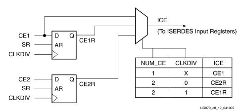
Figure 8-4: Input Clock Enable Module
