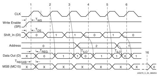
Figure 5-25: Slice SRL Timing Characteristics
