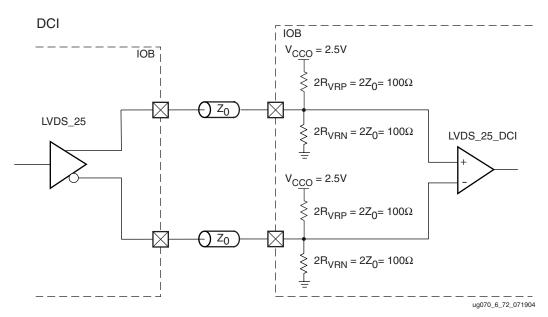
Figure 6-74: LVDS\_25\_DCI Receiver Termination
