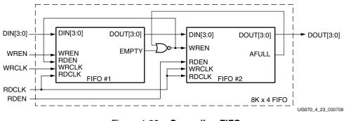
Figure 4-22: Cascading FIFO
