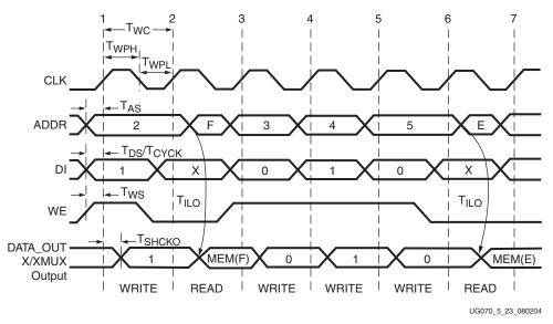
Figure 5-23: Slice Distributed RAM Timing Characteristics
