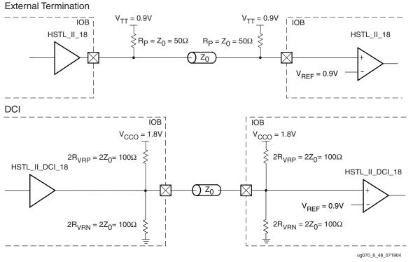
Figure 6-50: HSTL Class II (1.8V) with Unidirectional Termination
