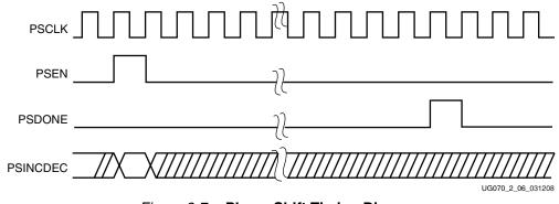
Figure 2-7: Phase-Shift Timing Diagram
