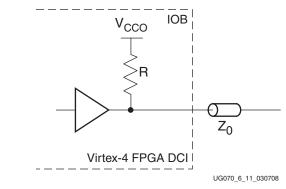
Figure 6-11: Driver with Termination to V<sub>CCO</sub> Using DCI Single Termination
