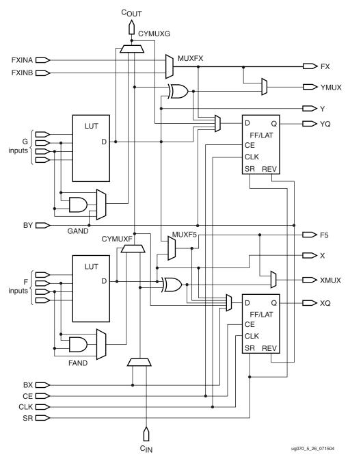
*Figure 5-26:* Simplified Virtex-4 FPGA Slice Carry-Chain Diagram
