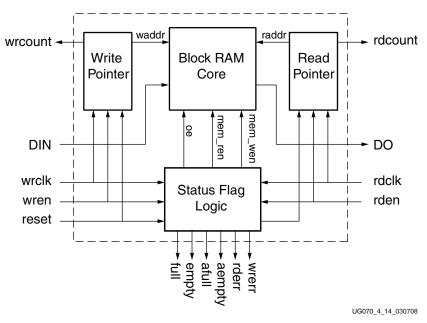
Figure 4-14: Top-Level View of FIFO in Block RAM
