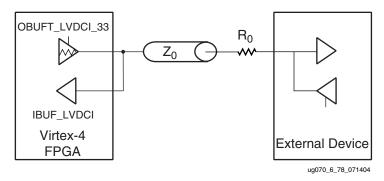
Figure 6-80: 3.3V I/O Configuration
