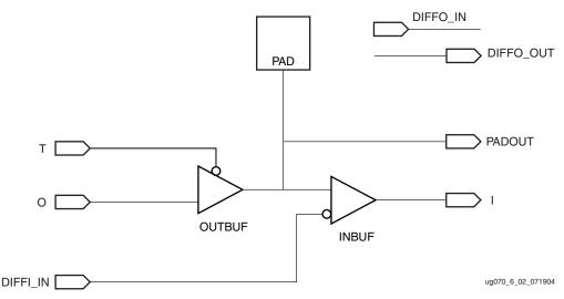
Figure 6-2: Basic IOB Diagram
