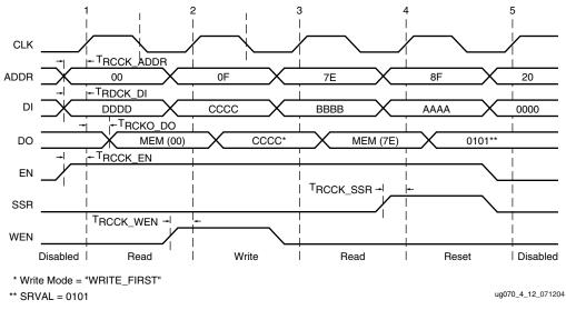
Figure 4-12: Block RAM Timing Diagram
