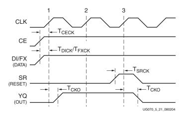
Figure 5-21 illustrates the general timing characteristics of a Virtex-4 FPGA slice.
