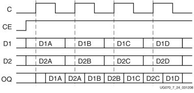
Figure 7-24: Output DDR Timing in SAME\_EDGE Mode
