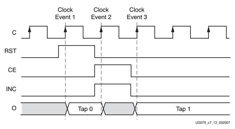
Figure 7-12 shows an IDELAY timing diagram. It is assumed that IOBDELAY\_VALUE = 0.
