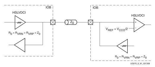
Figure 6-34: HSLVDCI Controlled Impedance Driver with Bidirectional Termination
