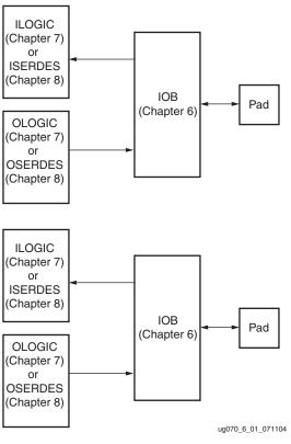
Figure 6-1: Virtex-4 FPGA I/O Tile
