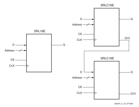
Figure 5-12: Simplified Shift Register and Cascadable Shift Register
