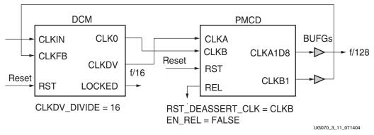
Figure 3-11: DCM to PMCD for Clock Frequency Division
