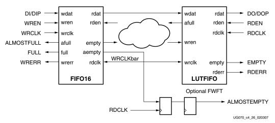
Figure 4-25: WRCLK Faster than RDCLK Design
