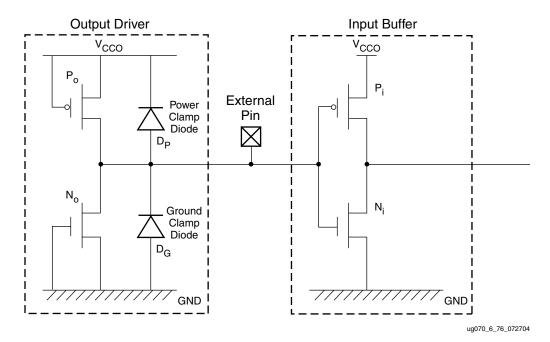
Figure 6-78: Virtex-4 FPGA I/O: 3-State Output Driver
