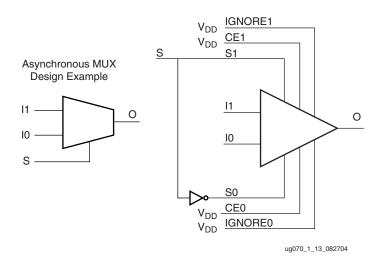
*Figure 1-13:* Asynchronous Mux with BUFGCTRL Design Example
