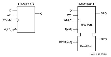
Figure 5-28: Single-Port and Dual-Port Distributed RAM Primitive
