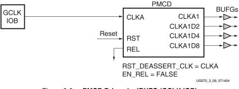
Figure 3-9: PMCD Driven by IBUFG (GCLK IOB)
