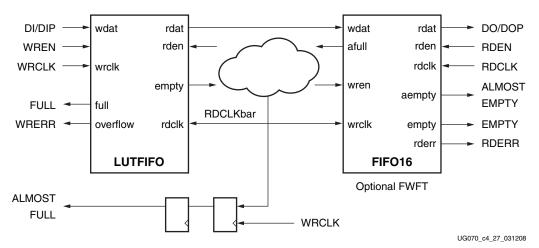
Figure 4-26: RDCLK Faster than WRCLK Design
