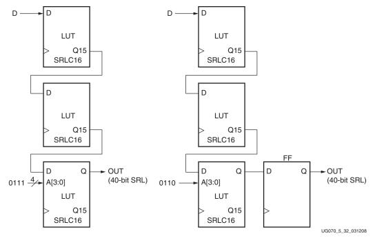
Figure 5-32: 40-bit Static-Length Shift Register
