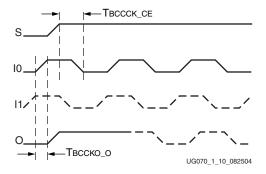
Figure 1-10: BUFGMUX\_1 Timing Diagram
