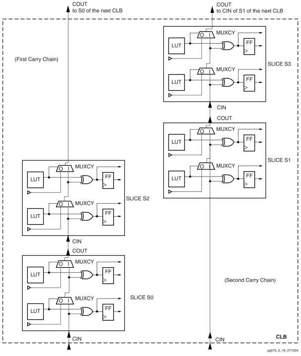
Figure 5-19: Fast Carry Logic Path
