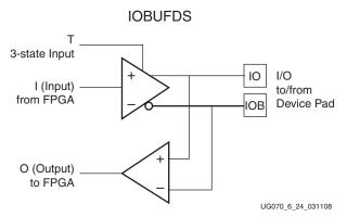
Figure 6-24: Differential Input/Output Buffer Primitive (IOBUFDS)
