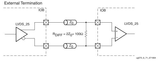
Figure 6-73: LVDS\_25 Receiver Termination
