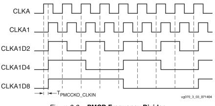
Figure 3-3: PMCD Frequency Divider
