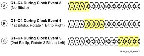
Figure 8-13: Bits from Data Input Stream (D) of Figure 8-12
