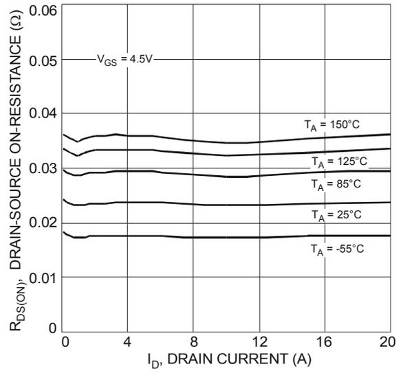
Fig. 4 Typical On-Resistance vs. Drain Current and Temperature
