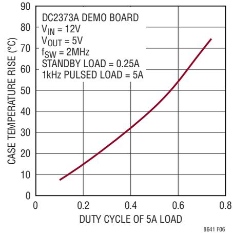
Figure 6. Case Temperature Rise vs 5A Pulsed Load
