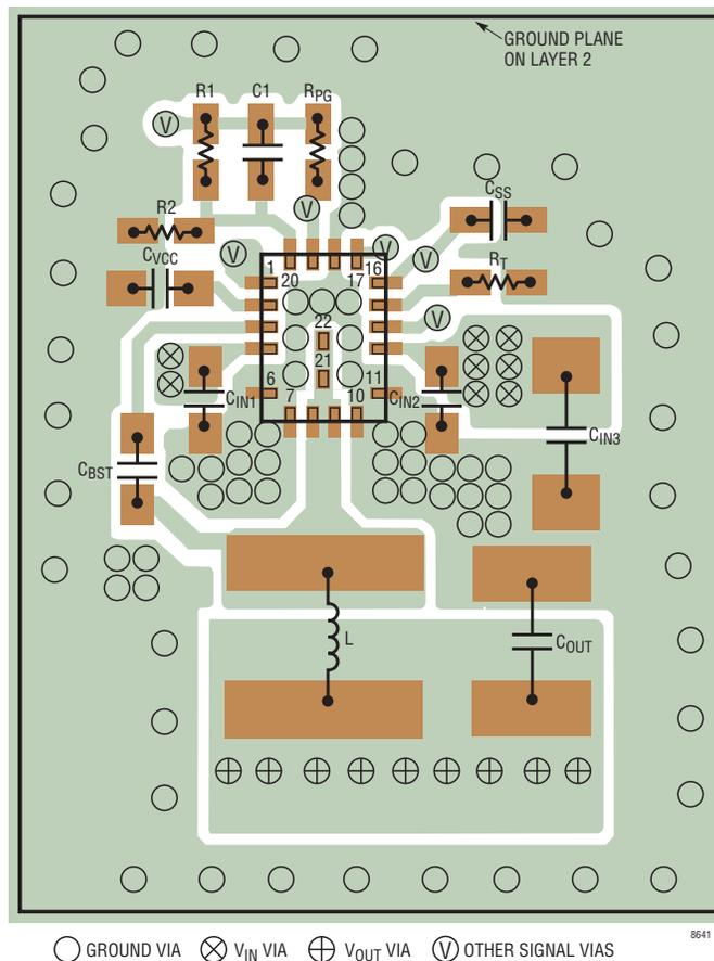
Figure 1. Recommended PCB Layout for the LT8641
