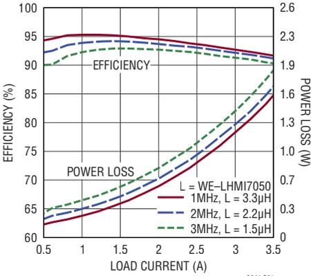
12V<sub>IN</sub> to 3.3V<sub>OUT</sub> Efficiency vs Frequency
