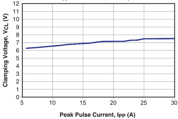
Clamping Voltage vs. Current
