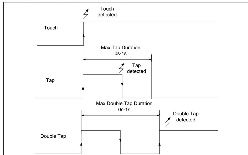
**FIGURE 2-49: TOUCH DETECTION – PARAMETERS ADJUSTMENT**
