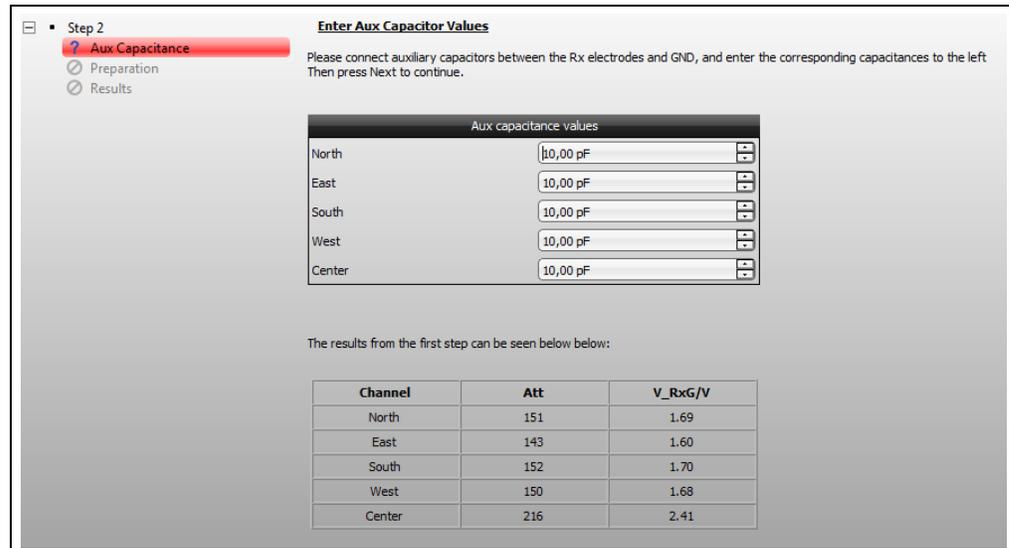
Pressing **Next** will show the Rx signal. The signal plot is generated by sweeping the sampling time, relative to the time instance when the Tx potential is switched to its high level. Electrode Capacitance Measurement uses the level at the sampling point indicated in [Figure 2-61](#) to calculate the  $V'_{RxG}$ . The Rx signal is generated at a working frequency of 115 kHz. The unit is digits.
