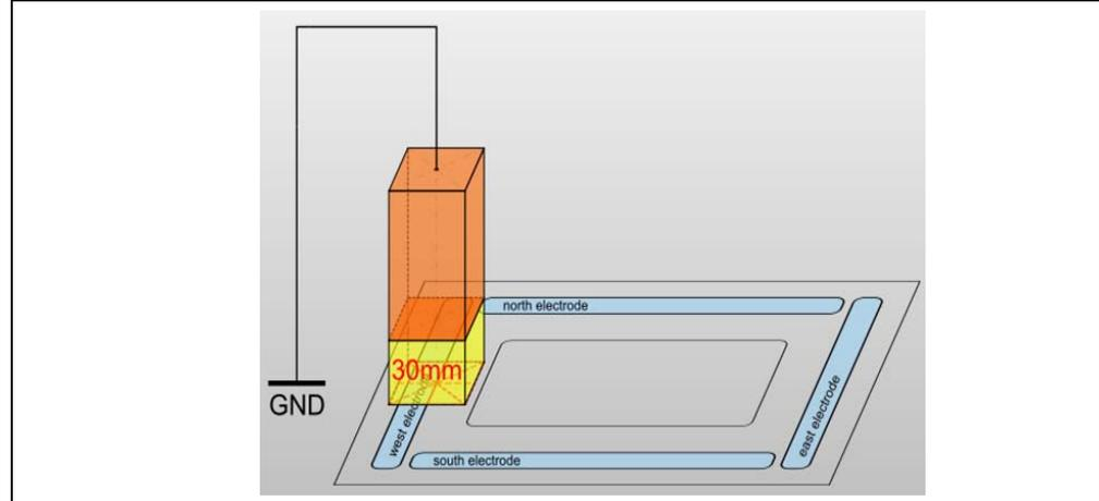
**Note:** It is not necessary to adjust or correct the 30 mm Styrofoam spacer brick for the thickness of the target device's housing or for a decoration layer covering the electrodes.
