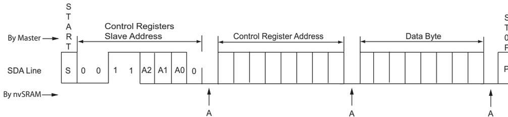
**Figure 23. Multi-Byte Write into Control Registers**
