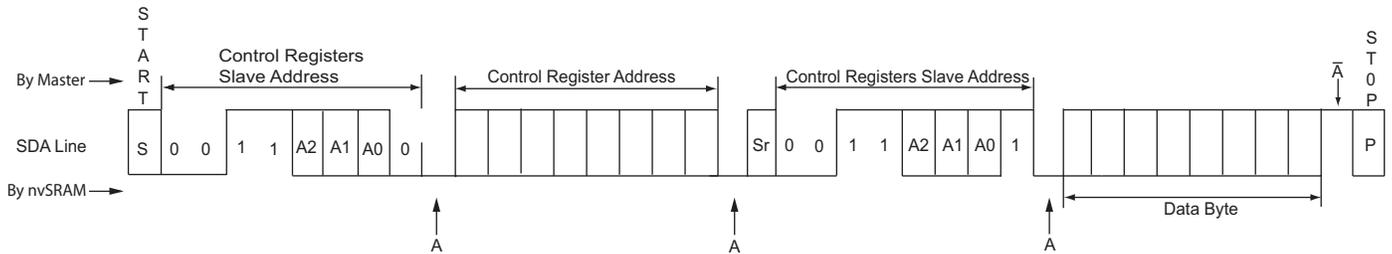
Figure 27. Random Control Registers Multi-Byte Read
