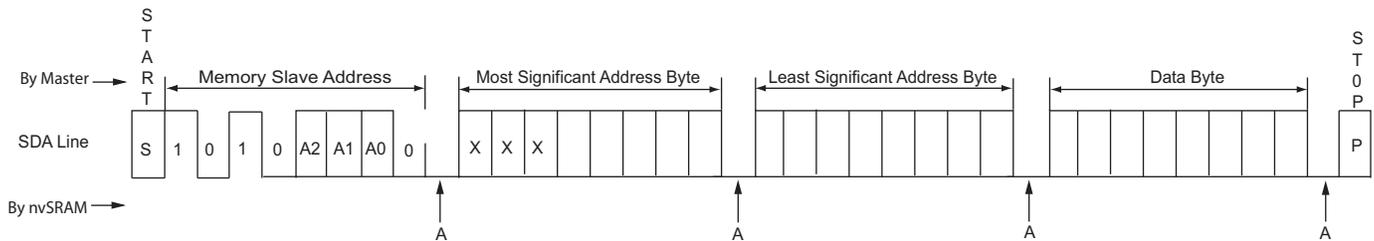
**Figure 11. Multi-Byte Write into nvSRAM (except Hs-mode)**
