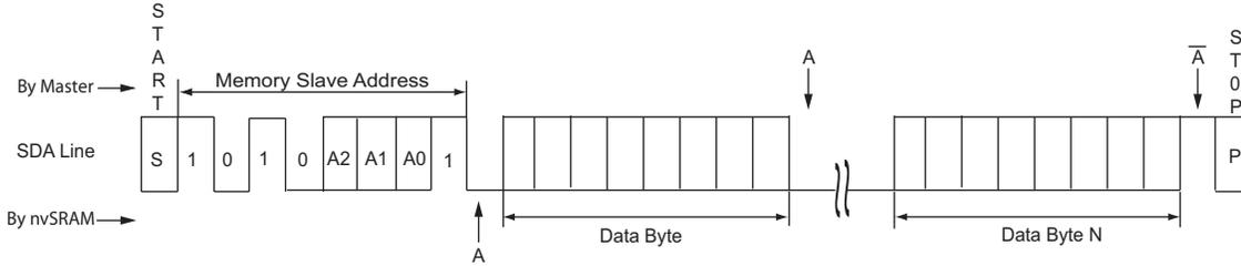
Figure 16. Current Location Single-Byte nvSRAM Read (Hs-mode)
