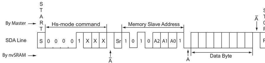
Figure 17. Current Location Multi-Byte nvSRAM Read (Hs-mode)
