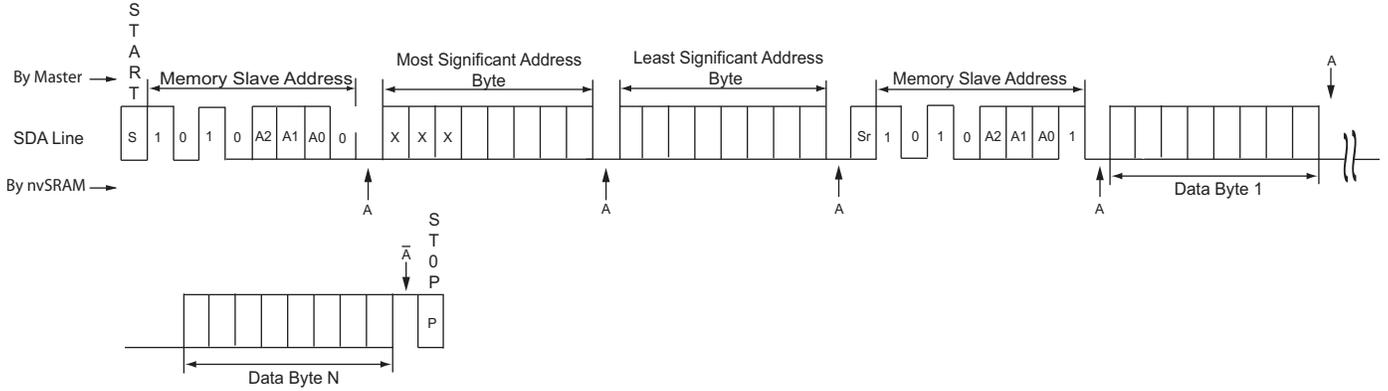
Figure 20. Random Address Single-Byte Read (Hs-mode)
