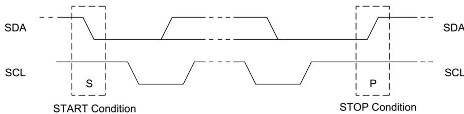
Figure 4. Data Transfer on the I<sup>2</sup>C Bus
