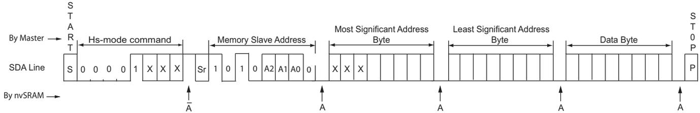
Figure 13. Multi-Byte Write into nvSRAM (Hs-mode)
