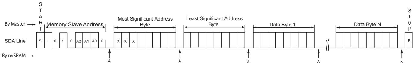
Figure 12. Single-Byte Write into nvSRAM (Hs-mode)
