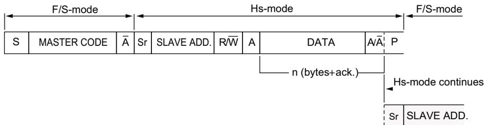
Single and multiple-byte reads and writes are supported. After the device enters Hs-mode, data transfer continues in Hs-mode until the stop condition is sent by the master device. The slave switches back to F/S-mode after a STOP condition (P). To continue data transfer in Hs-mode, the master sends Repeated START (Sr).
