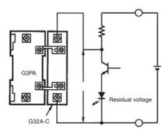
In rated operation, the G3PA turns ON at 4 V max. Ordinarily, the G3PA might turn ON if the residual voltage in transistor circuits exceeds 3 V. (The G32A-C makes voltage output at voltages exceeding 9.6 V.)
