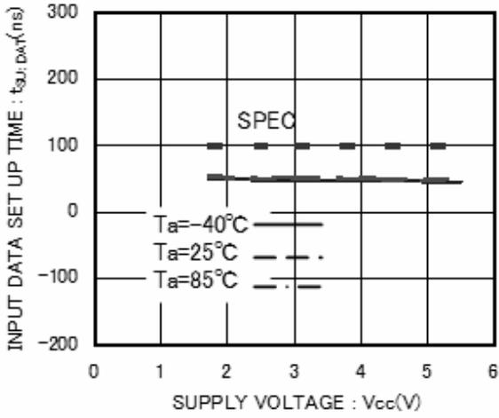
Figure 18. Input Data Setup Time  $t_{SU:DAT}$  (HIGH)
