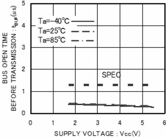
Figure 22. BUS open time before transmission  $t_{BUF}$
