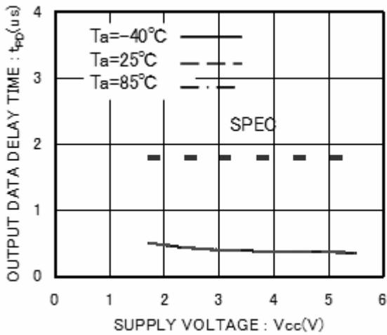
Figure 20. "L" Data output delay time  $t_{PD0}$
