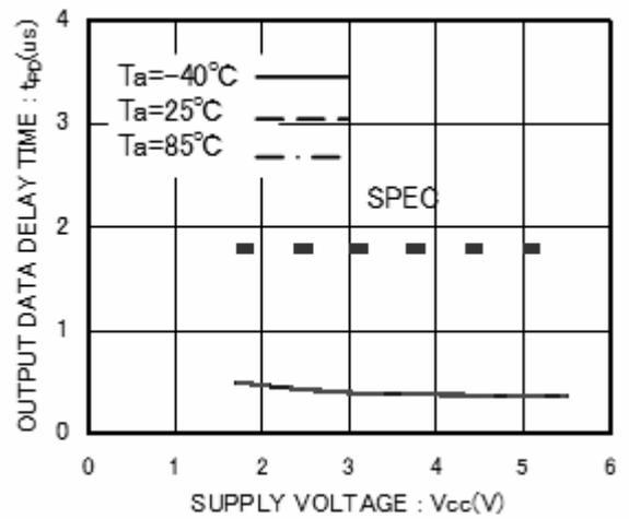
Figure 21. 'H' Data output delay time  $t_{PD1}$
