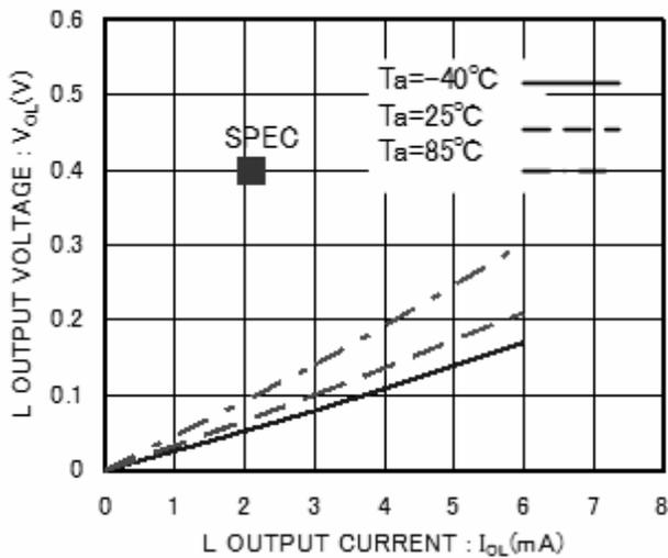
Figure 4. 'L' output voltage  $V_{OL} - I_{OL}$  ( $V_{CC}=1.7$ )
