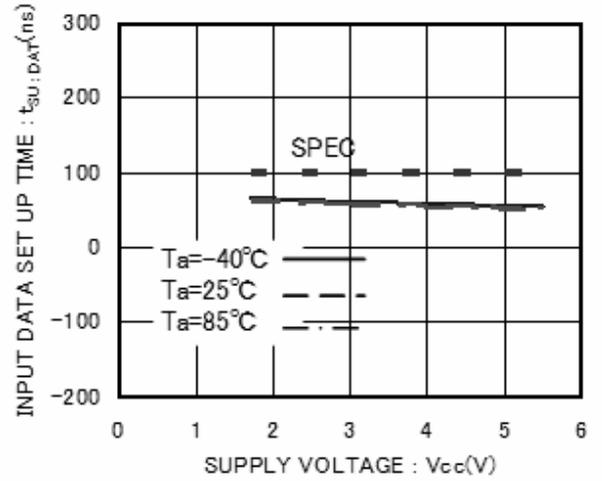
Figure 19. Input Data Setup Time  $t_{SU:DAT}$  (LOW)
