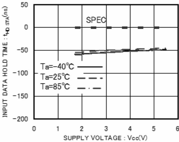
Figure 16. Input Data Hold Time  $t_{HD:DAT}$  (HIGH)
