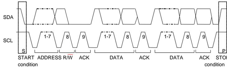
Figure 30. Data transfer timing
