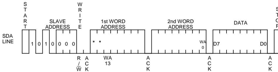
Figure 31. Byte write cycle
