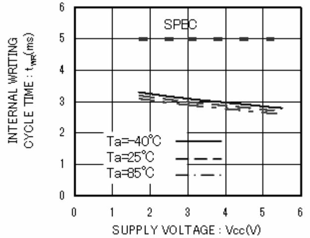
Figure 23. Internal writing cycle time  $t_{WR}$
