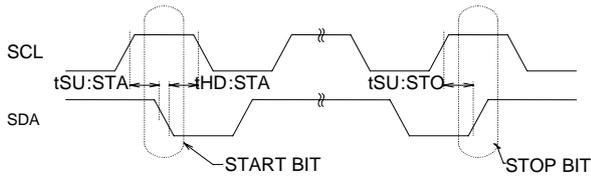
Figure 1-(b) Start - stop bit timing
