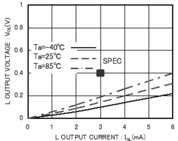
Figure 5. 'L' output voltage  $V_{OL} - I_{OL}$  ( $V_{CC}=2.5V$ )
