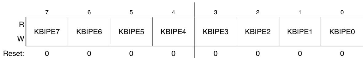
Figure 7-3. KBI Pin Enable Register (KBIPE)
