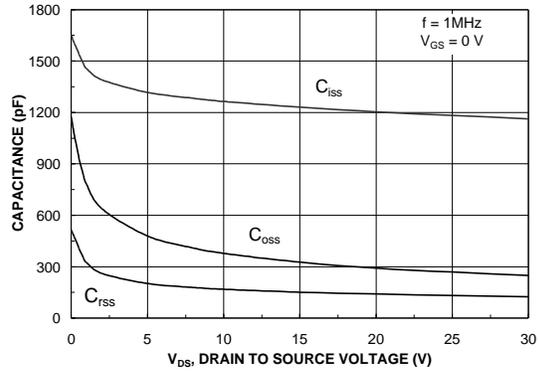
Figure 8. Capacitance Characteristics
