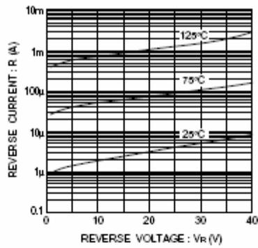
Fig. 2 Reverse characteristics
