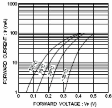
Fig. 1 Forward characteristics
