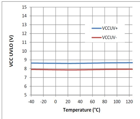
**Figure 24.** V<sub>CC</sub> UVLO vs. Temperature
