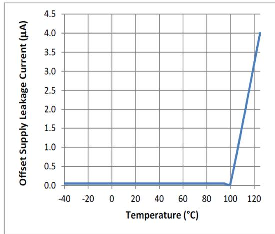
**Figure 25.** Offset Supply Leakage Current vs. Temperature
