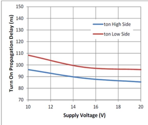
**Figure 4.** Turn-on Propagation Delay vs. Supply Voltage
