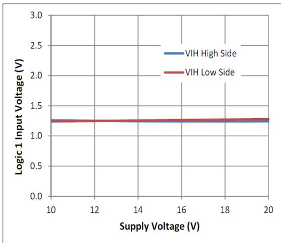
**Figure 20.** Logic 1 Input Voltage vs. Supply Voltage
