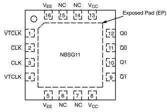
Figure 1. BGA-16 and LGA-16 Pinout (Top View)
