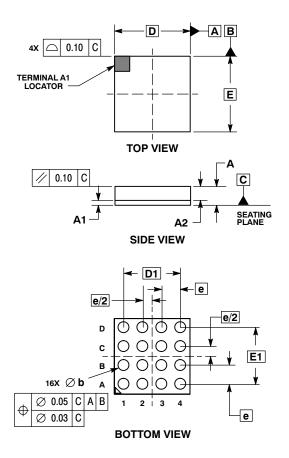
NOTES: 1. DIMENSIONING AND TOLERANCING PER ASME Y14.5M, 1994. 2. CONTROLLING DIMENSION: MILLIMETERS.
