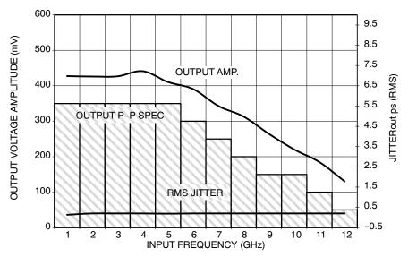
Figure 4. Output Voltage Amplitude (V<sub>OUTPP</sub>) / RMS Jitter vs. Input Frequency (f<sub>in</sub>) at Ambient Temperature (Typical)
