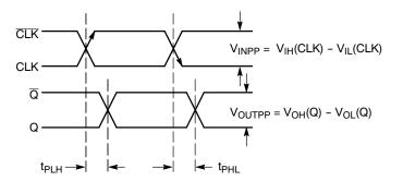
Figure 5. AC Reference Measurement
