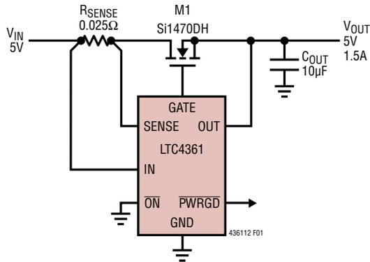
Figure 1. Protection from Input Overvoltage and Overcurrent
