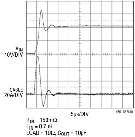
Figure 4. 20V Hot-Plug into a 10µF Capacitor
