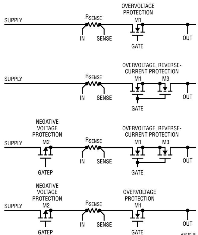
Figure 3. MOSFET Configurations
