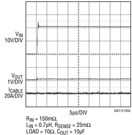
Figure 5. 20V Hot-Plug into the LTC4361
