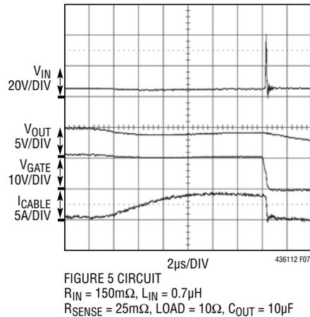
Figure 7. Overcurrent Turn-Off and Resulting Input Transient
