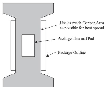
Layout recommendations for a Single Layer PCB: utilize as much Copper Area for Power Management. In a single layer board application the thermal pad is attached to a heat spreader (copper areas) by using low thermal impedance attachment method (solder paste or thermal conductive epoxy).
