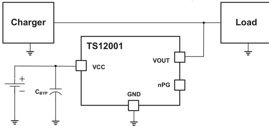
Note: When the TS12001 is Off-Active™, the battery will continue to charge through the body diode between VOUT and VCC.
