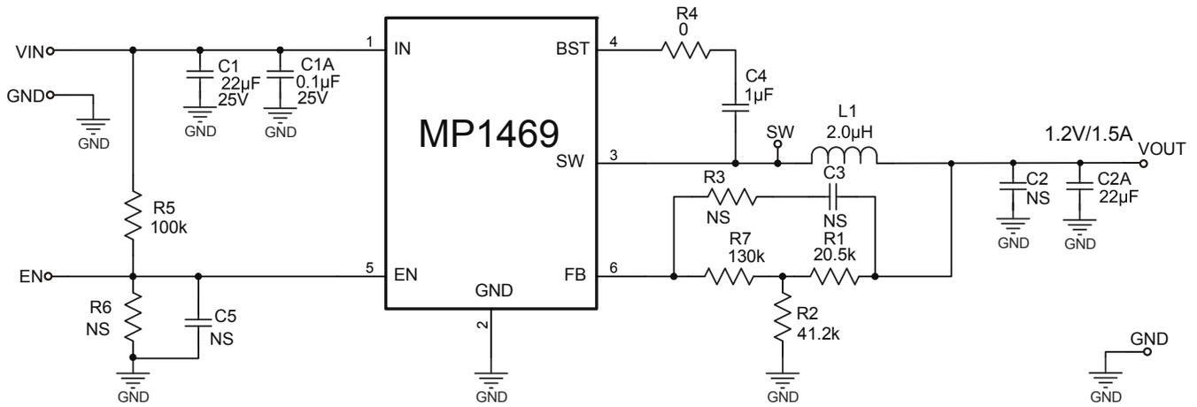
**Figure 12: 12V<sub>IN</sub>, 1.2V/1.5A**
