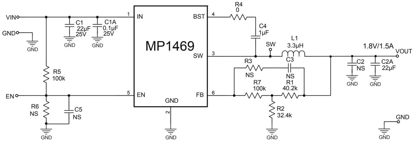
**Figure 11: 12V<sub>IN</sub>, 1.8V/1.5A**
