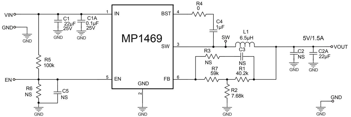
**Figure 8: 12V<sub>IN</sub>, 5V/1.5A**
