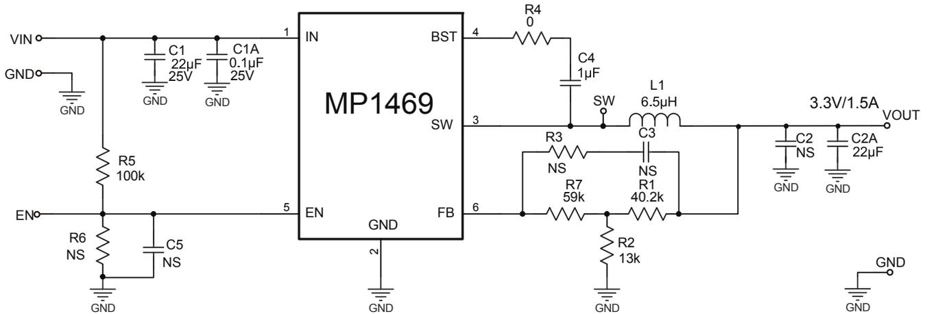
**Figure 9: 12V<sub>IN</sub>, 3.3V/1.5A**
