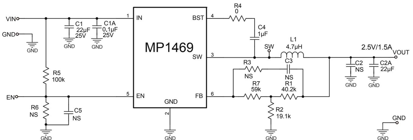
**Figure 10: 12V<sub>IN</sub>, 2.5V/1.5A**
