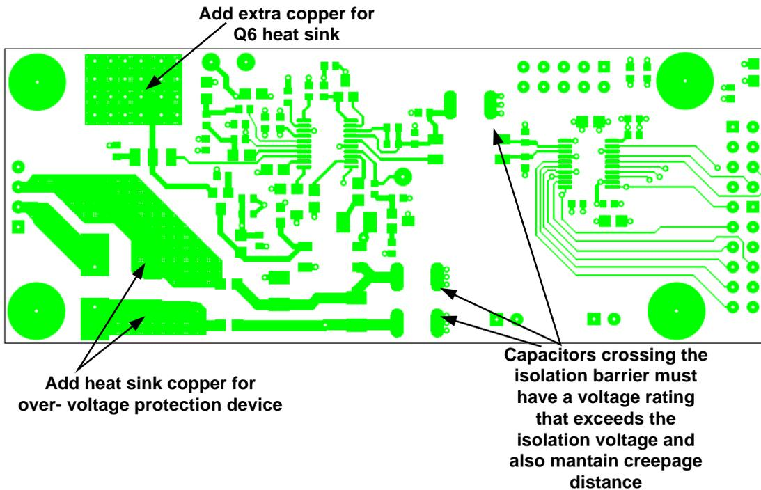
Figure 7: 73M1966B Reference PCB Top Copper Layer
