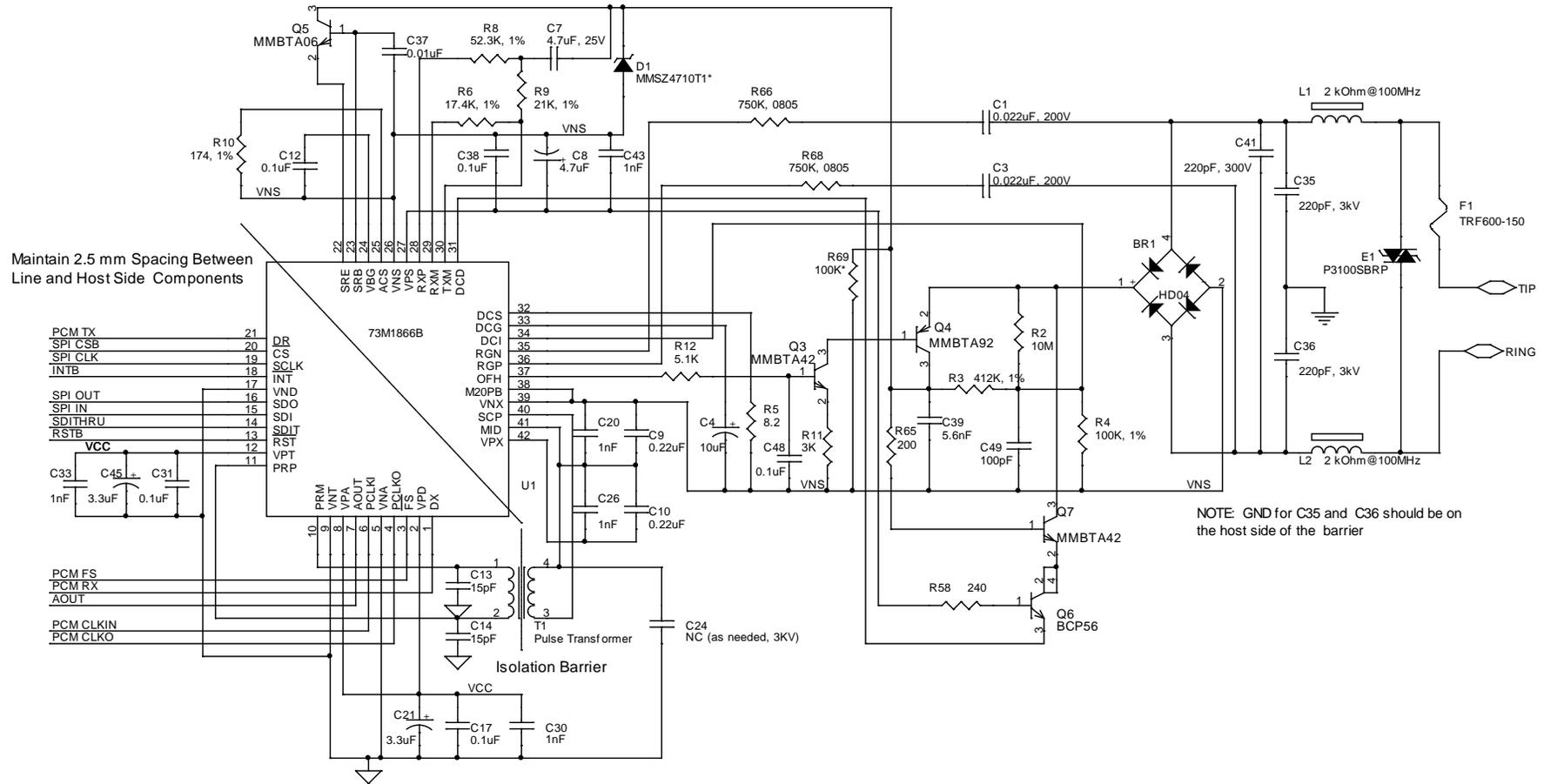
Figure 5: 73M1866B Reference Schematic
