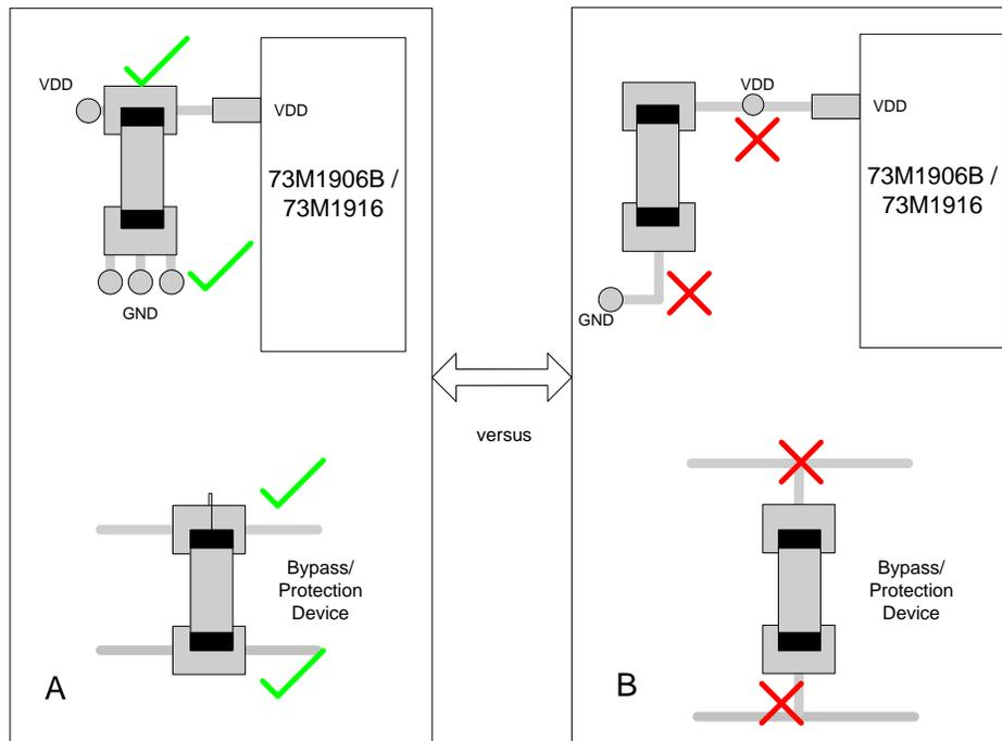
**Figure 3: Layout and Routing of Power/Bypass Capacitors**
