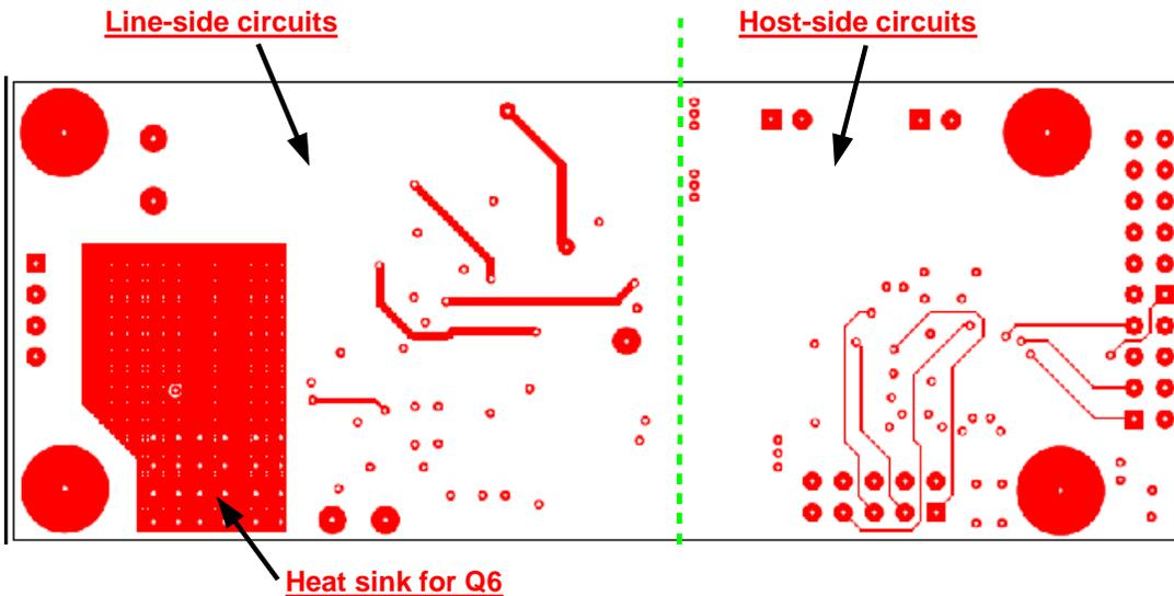
Figure 8: 73M1966B Reference PCB Bottom Copper Layer
