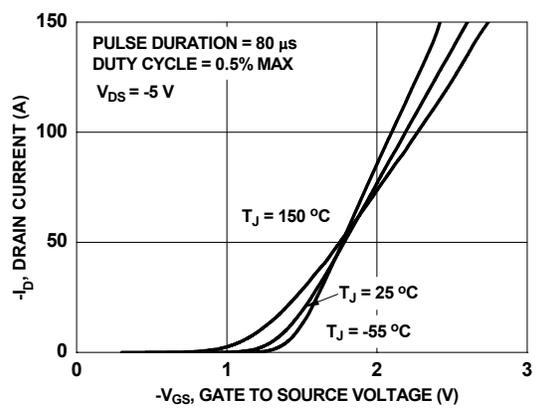
**Figure 5. Transfer Characteristics**
