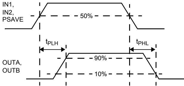
Figure 4.  $t_{PLH}$  and  $t_{PHL}$  Timing
