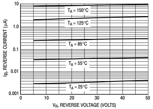
Figure 3. Leakage Current
