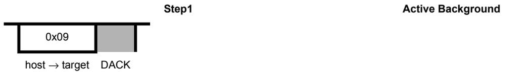
This command is used to step through application code. In active BDM, this command executes the next CPU instruction in application code. If enabled an ACK is driven.
