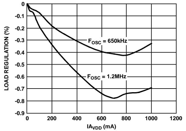
FIGURE 2. A<sub>VDD</sub> LOAD REGULATION vs I<sub>A<sub>VDD</sub></sub>
