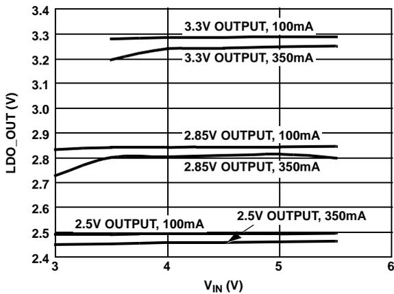
FIGURE 5. LINE REGULATION LDO\_OUT vs V<sub>IN</sub>
