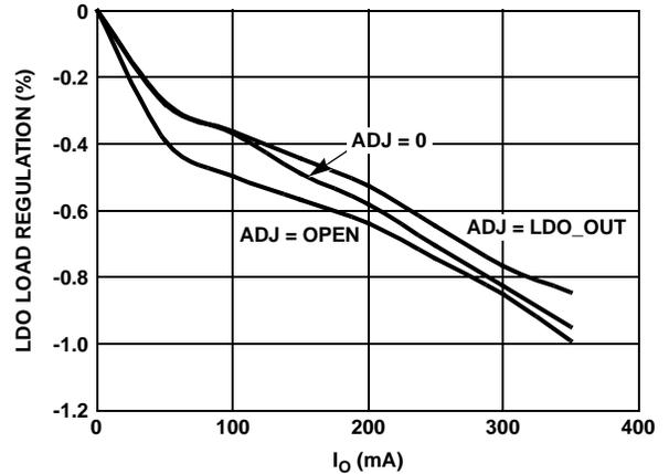
FIGURE 6. LDO LOAD REGULATION vs I<sub>O</sub>
