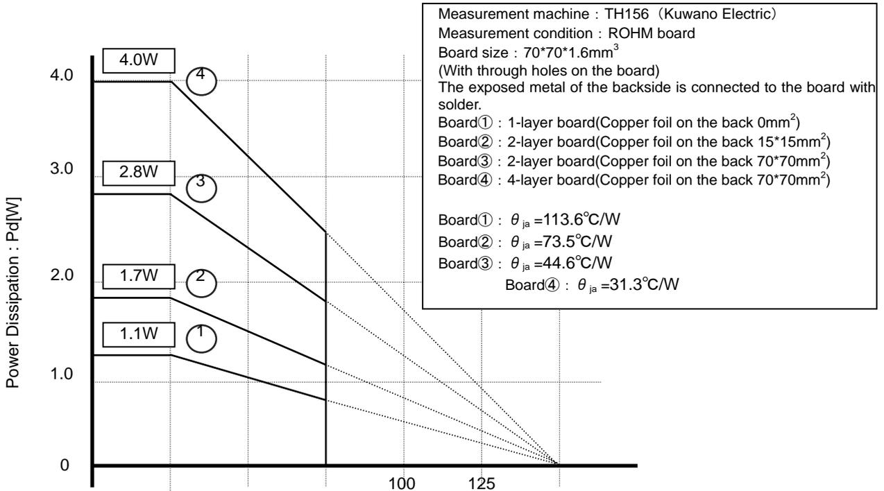
Fig.2 HTSSOP-B24 Derating curve
