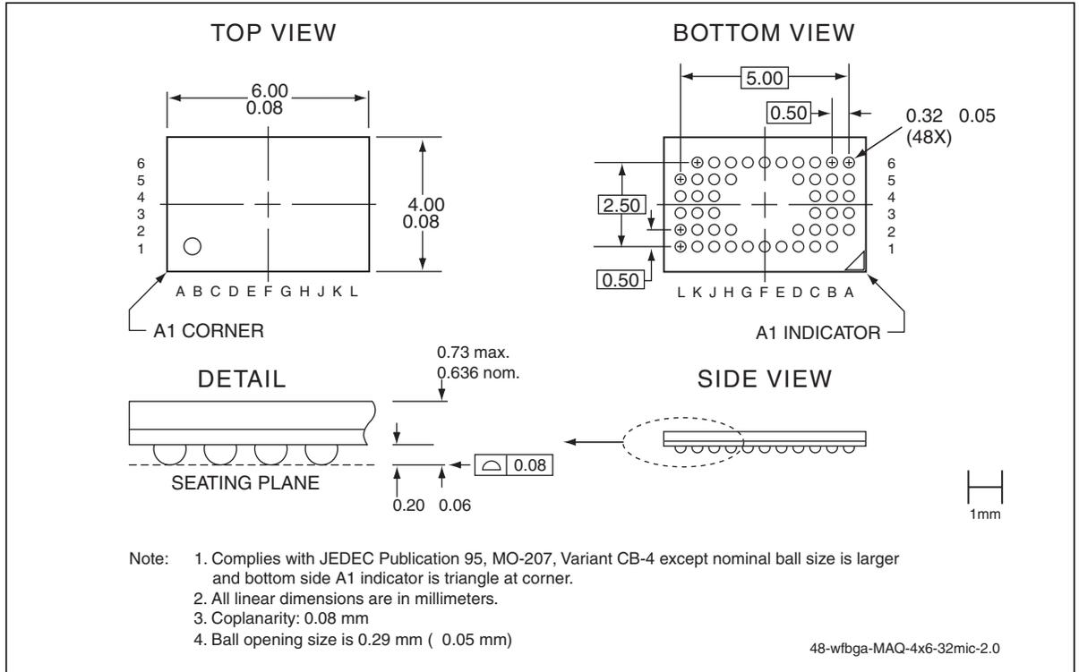
**Figure 29:**48-ball Very, Very Thin-profile, Fine-pitch Ball Grid Array (WFBGA) 6mm x 8mm
