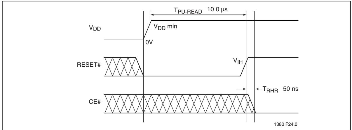
Figure 5: Power-Up Diagram
