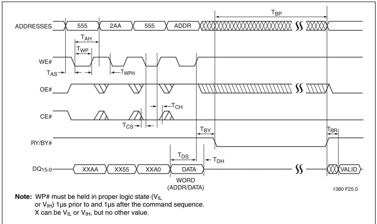
**Figure 7:** WE# Controlled Program Cycle Timing Diagram
