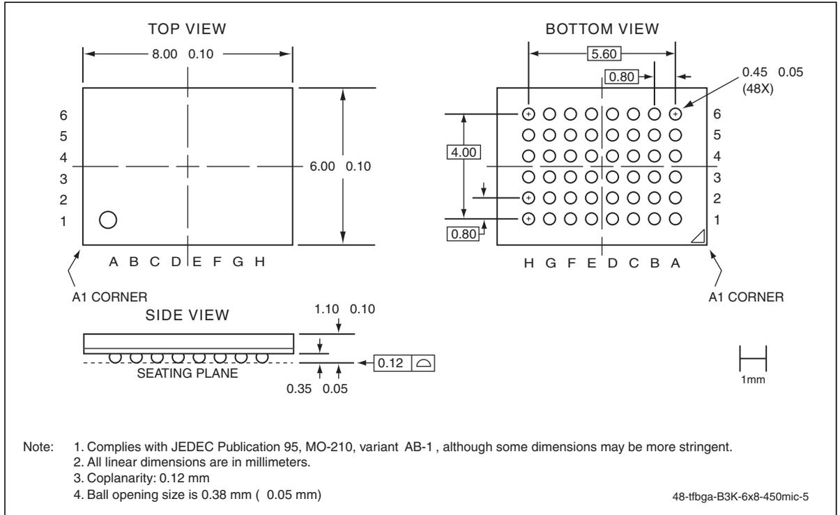
**Figure 28:**48-ball Thin-profile, Fine-pitch Ball Grid Array (TFBGA) 6mm x 8mm
