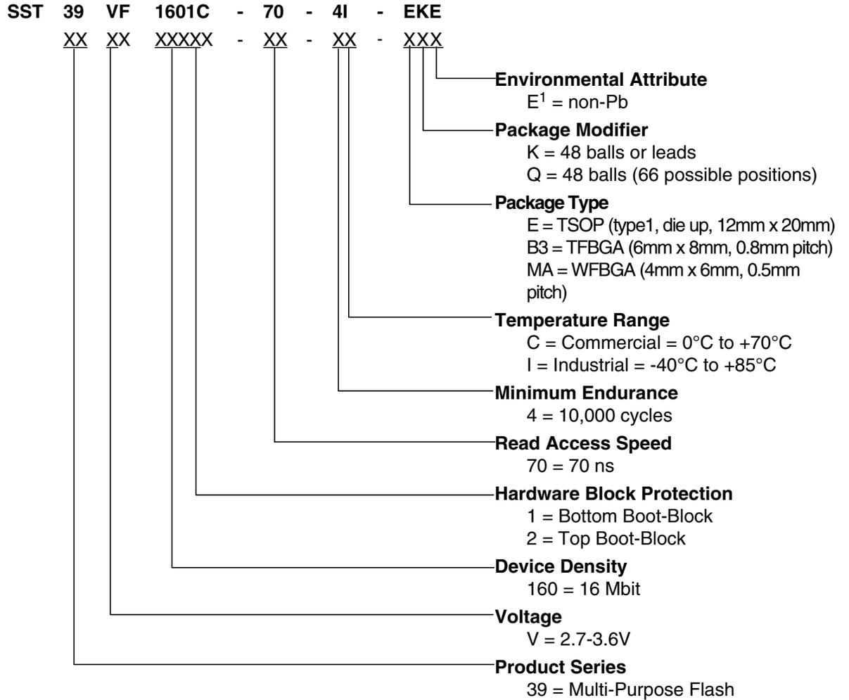
1. Environmental suffix "E" denotes non-Pb solder. SST non-Pb solder devices are "RoHS Compliant".
