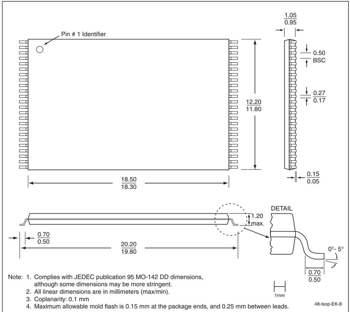
**Figure 27:**48-lead Thin Small Outline Package (TSOP) 12mm x 20mm
