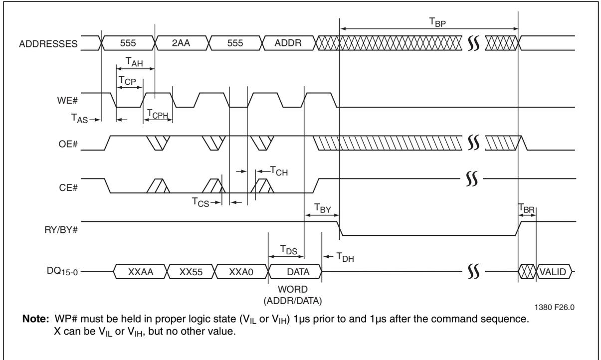
**Figure 8:** CE# Controlled Program Cycle Timing Diagram
