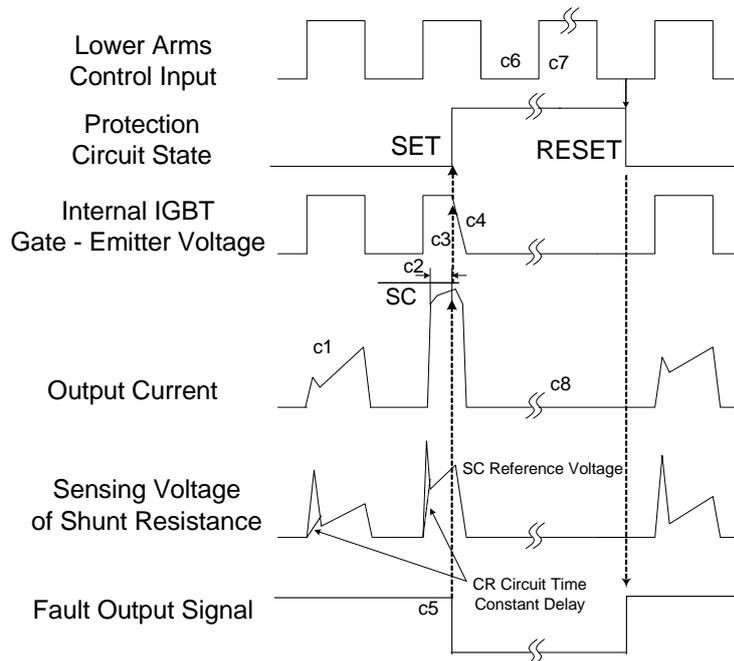
**Figure 13. Short-Circuit Protection (Low-Side Operation Only)**
