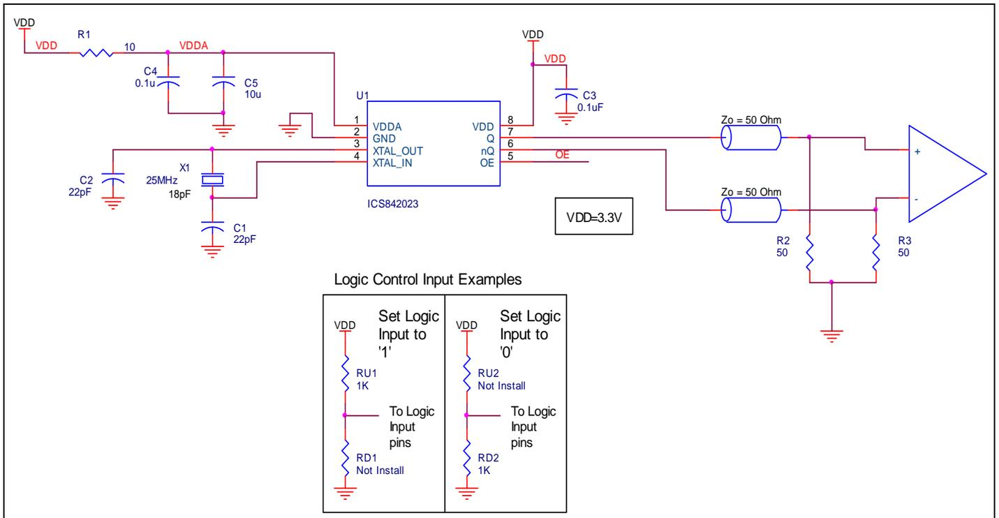
Figure 5. 842023 Schematic Example
