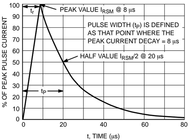
Figure 5. 8 × 20 μs Pulse Waveform
